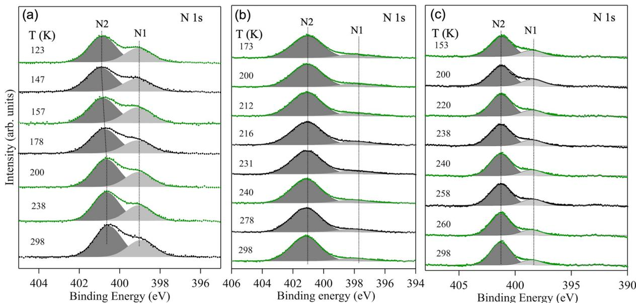
Fig. 3 Temperature dependent XPS of the N 1s core-level of (a)  $\text{Fe}(\text{phen})_2(\text{NCS})_2$ , (b)  $[\text{Fe}(\text{3-Fpy})_2\{\text{Ni}(\text{CN})_4\}]$ , and (c)  $[\text{Fe}(\text{3-Fpy})_2\{\text{Pt}(\text{CN})_4\}]$ . As in Fig. 2, the raw spectra in green depict lowering of temperature while the ones in black represent increase in temperature.
