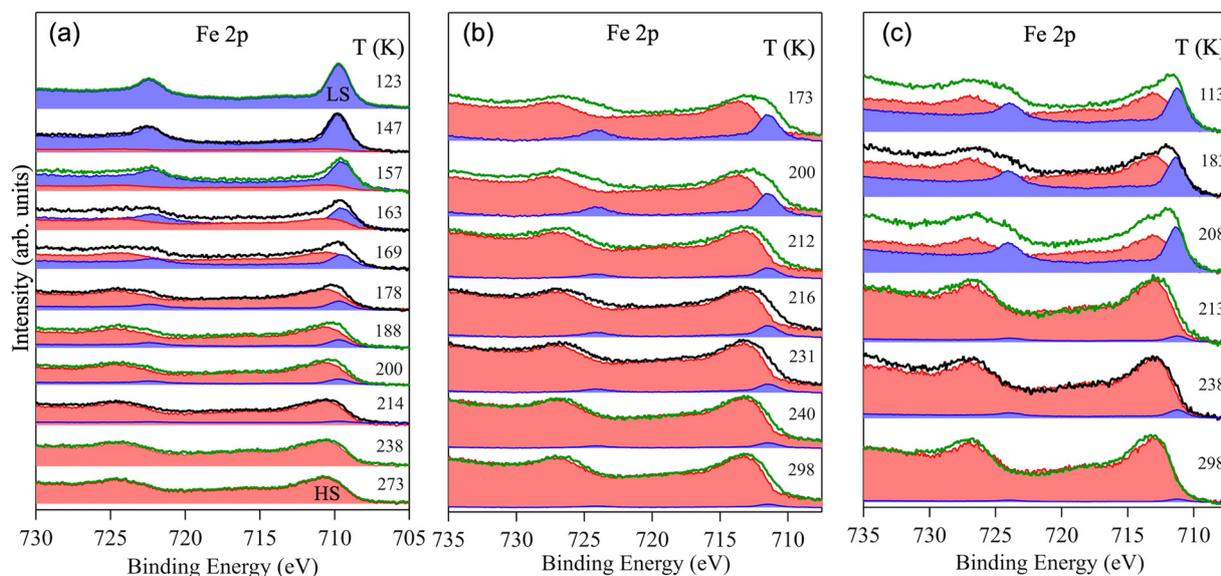
Fig. 2 Temperature dependent XPS of the Fe 2p core-level of (a)  $Fe(phen)_2(NCS)_2$ , (b)  $[Fe(3-Fpy)_2\{Ni(CN)\}_4]$ , and (c)  $[Fe(3-Fpy)_2\{Pt(CN)\}_4]$ . The raw spectra in green depict lowering of temperature while the ones in black represent increase in temperature. The fits in blue indicate the LS, and the fits in red represent the HS.
