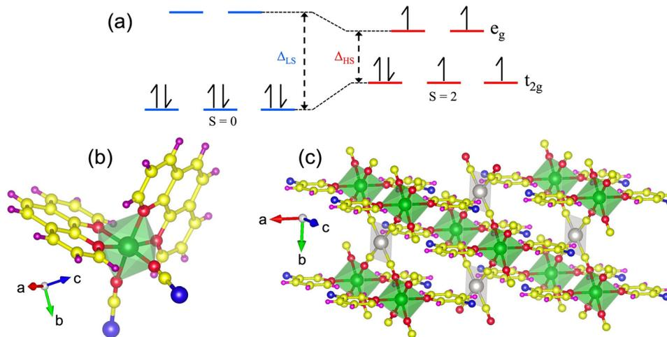
Fig. 1 (a)  $[Ar]3d^6$  electronic configuration in an octahedral ligand field of the Fe(II) ion in the LS and HS states, and ball-and-stick models of (b)  $Fe(phen)_2(NCS)_2$  and (c) the Hofmann-like Fe(II) SCO complexes, respectively. Atom codes for Fig. 1b: Fe (green); N (red); C (yellow); S (blue); H (purple). Atom codes for Fig. 1c: Fe (green); Ni/Pt (silver); N (red); C (yellow); F (blue); H (purple).
