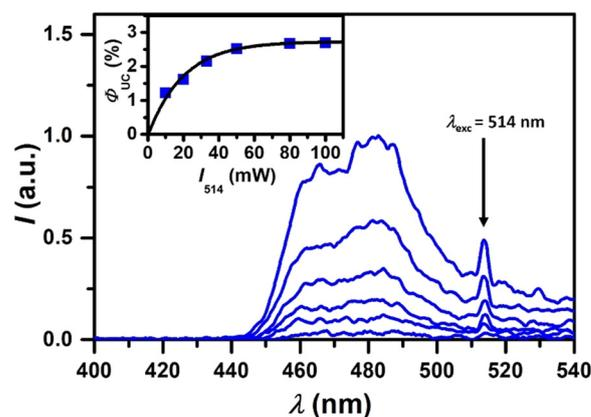
Fig. 5 Photon upconversion studies of 28  $\mu\text{M}$  BDP-Br and 100  $\mu\text{M}$  TBPe in deaerated ACN using a 514 nm cw laser for excitation. Main plot: UC Emission spectra with increasing laser intensity. Inset: the external UC quantum yield plotted against the laser intensity. See the text and ESI $^\dagger$  for details.
