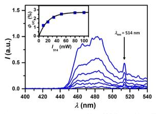
Fig. 5 Photon upconversion studies of 28 μM BDP-Br and 100 μM TBPe in deaerated ACN using a 514 nm cw laser for excitation. Main plot: UC Emission spectra with increasing laser intensity. Inset: the external UC quantum yield plotted against the laser intensity. See the text and ESI† for details
