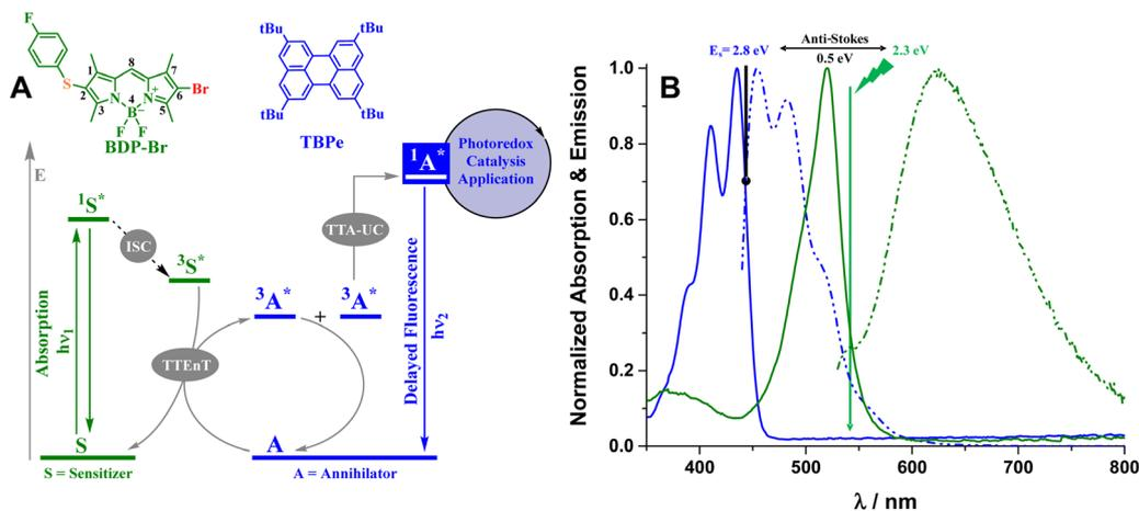
**Fig. 1** (A): Schematic representation of the corresponding photophysical events associated with the TTA-UC phenomenon enabled by the **BDP-Br** (sensitizer) and **TBPe** (annihilator) pair and its implementation in photoredox catalysis. (B): Normalized absorption (solid line) and emission (dashed dotted line) spectra of **BDP-Br** (green) and **TBPe** (blue) in 8  $\mu\text{M}$  aerated acetonitrile/dimethylacetamide (4/1 v/v) solution.
