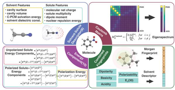
Fig. 1 Diagram of four types of descriptors for solvated molecules.
