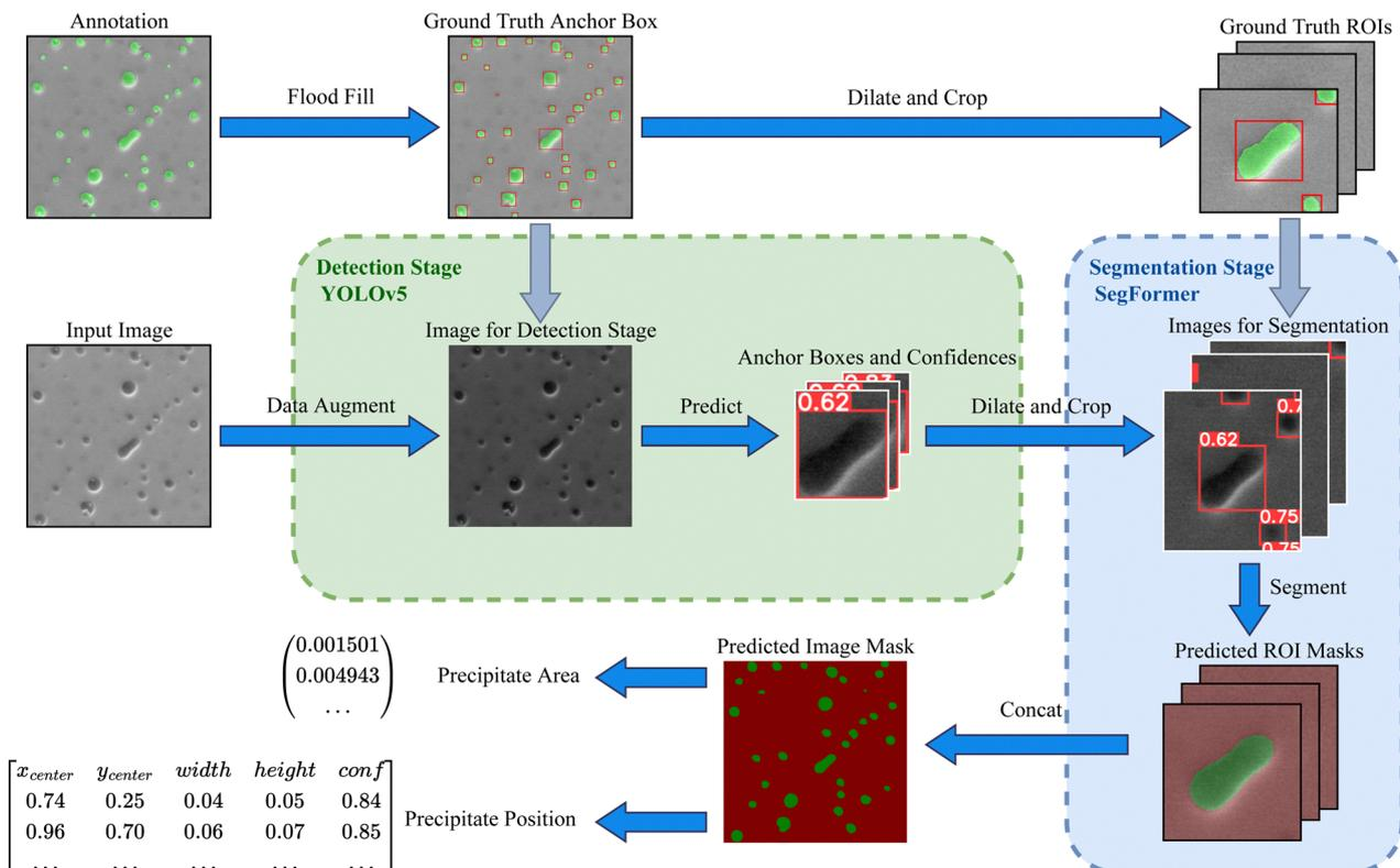
Fig. 2 Architecture and pipeline of the proposed DT-SegNet. The first step is to pre-process the input image to fit the input size of the detection network. Once predicted, the anchor boxes are dilated and cropped before feeding into the segmentation network. Finally, the accurate mask, area and position of precipitate objects are derived.
