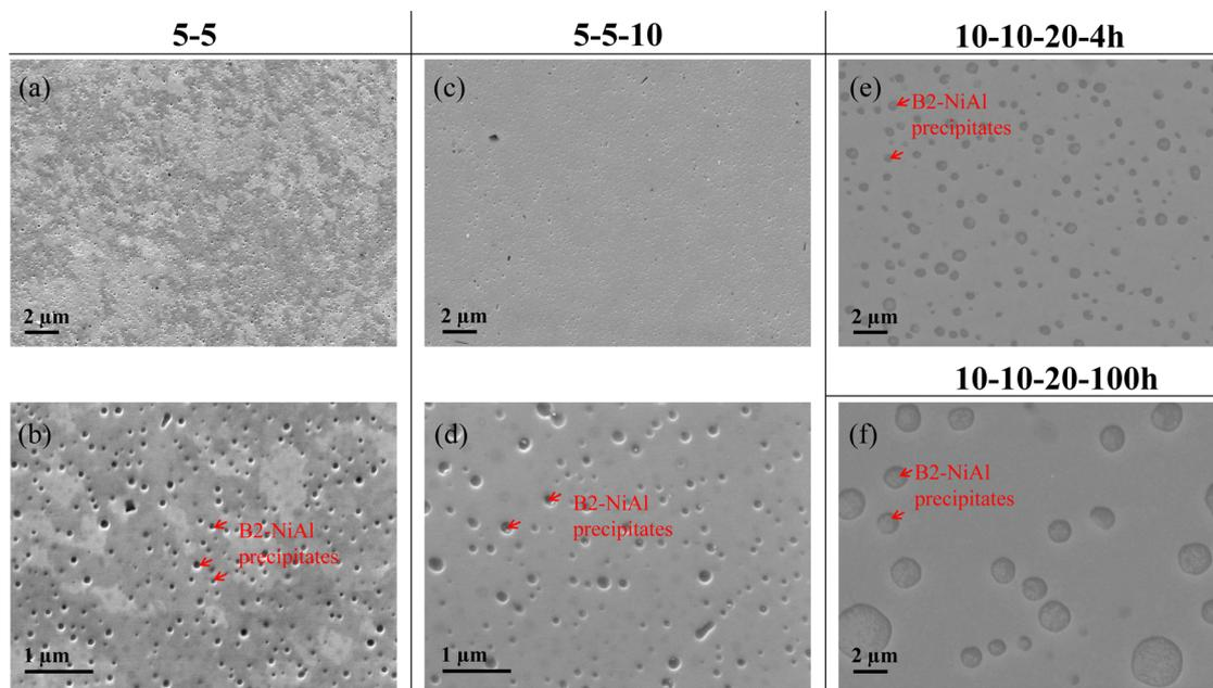
**Fig. 1** SEM micrographs showing the general microstructure of (a) Cr-5Ni-5Al, (c) Cr-5Ni-5Al-10Fe, (e) and (f) Cr-10Ni-10Al-20Fe aged differently. (b) and (d) are zoomed images respectively of (a) and (c).
