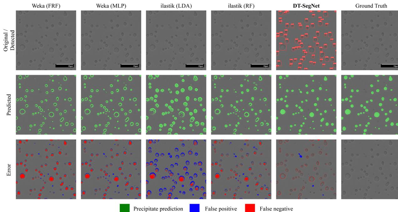
Fig. 10 Visualisation of segmentation results on 10-10-20-100 h produced by four competing methods and this study's methods, along with the ground truth annotation.
