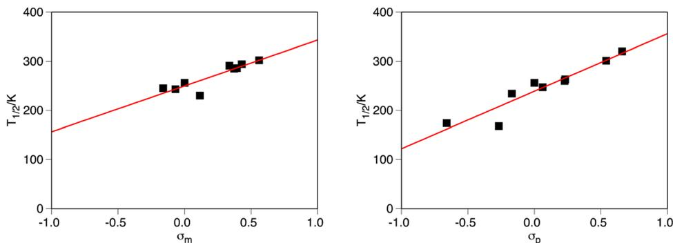
Fig. 2 Correlation between the computed  $T_{1/2}$  with the Sigma Hammett constants for the  $[\text{Fe}(\text{L}_2^{\text{R}p/\text{R}m})(\text{im})_2]^+$  ( $\text{R} = -\text{NH}_2, -\text{OMe}, -\text{F}, -\text{Cl}, -\text{Br}, -\text{CH}_3, -\text{H} -\text{CN}$  and  $-\text{CH}_3$ ) system. Left,  $\text{L}_2^{\text{R}m}$  and right  $\text{L}_2^{\text{R}p}$  ligands ( $R^2 = 0.79$  and  $0.88$ , respectively).
