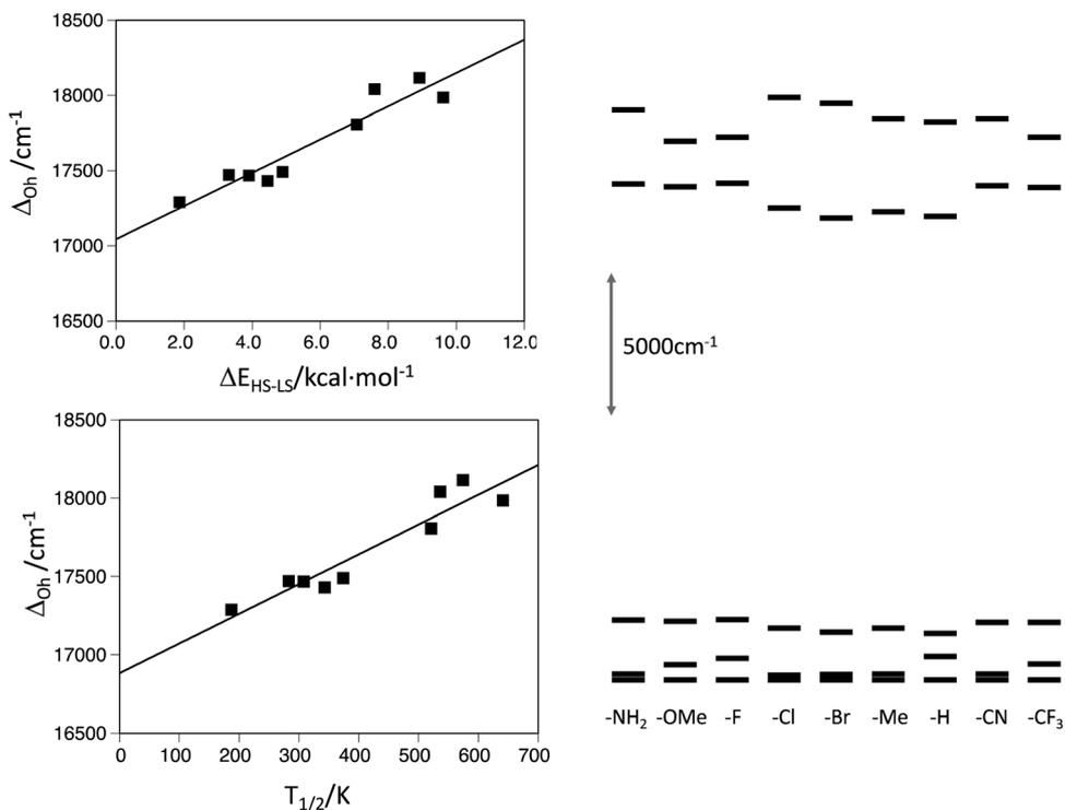
Fig. 5 Left, correlations between the computed d-MOs splitting and the spin-state energy gap ( $\Delta E_{\text{HS-LS}}$ ) and computed transition temperature ( $T_{1/2}$ ) of  $[\text{Fe}(L_1^R)(\text{im})_2]^+$ . Right, energy of the five d-MOs extracted from the *ab initio* ligand field theory applied to the NEVPT2 calculation on the low-spin ( $S = 1/2$ ) optimized geometry. ( $R^2$  values are  $0.84$  and  $0.89$ , respectively).
