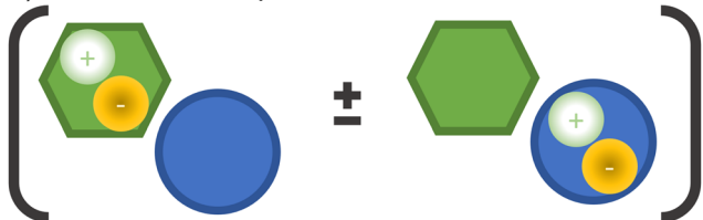
Fig. 8 Types of electronic energy transport. In the schemes, the hexagon and the circle represent different chromophores. (a) FRET: a localized exciton in one chromophore is transferred to the other through energy resonance (indicated by the virtual photon, h\nu ). (b) Dexter energy transfer: a localized exciton is transferred at short distances via electron exchange between the chromophores (indicated by the electron, e^- , and electron-hole, h^+ , transfers). (c) Coherent transport: an entangled quantum exciton is formed over the chromophores. The transport occurs when the electronic wave function collapses to a localized excitation. Although the diagrams illustrate neighbor chromophores, they can be far from each other in FRET and coherent transport.
