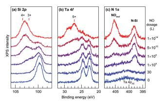
Fig. 3 (a) Si 2p, (b) Ta 4f, and (c) N 1s core level XPS spectra for Ta@Si $_{16}$  deposited on a C $_{60}$  substrate before and after step by step exposure to NO. Reproduced from ref. 109 with permission from the Royal Society of Chemistry.
