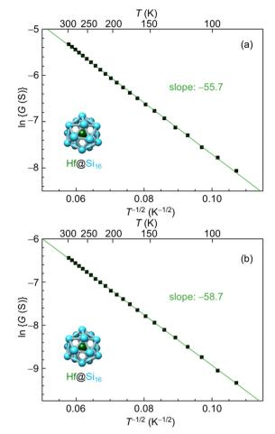
Fig. 9 Temperature dependent electrical conductance of a Hf@Si $_{16}$  assembled film based on the ES-VRH model; (a) as deposition and (b) after annealing at 423 K for 90 min in a vacuum. The logarithm of conductance (ln *G*) versus  $T^{-1/2}$  for Hf@Si $_{16}$  films is plotted at 87–300 K, and the slope values are shown in each.
