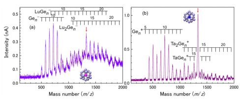
Fig. 5 Mass spectra for M-Ge binary NC anions of (a) M = Lu and cations of (b) M = Ta. Red arrows indicate the peak corresponding to  $M@Ge_{16}^{\pm}$ .
