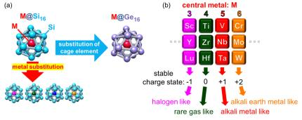
Fig. 1 Overview of  $M@Si_{16}$  and  $M@Ge_{16}$  SAs. (a) Geometric structure of  $M@Si_{16}$  with metal substitution and cage element substitution into  $M@Ge_{16}$ . (b) Transition metal to be encapsulated and the corresponding superatomic nature of  $M@Si_{16}$  and  $M@Ge_{16}$ .
