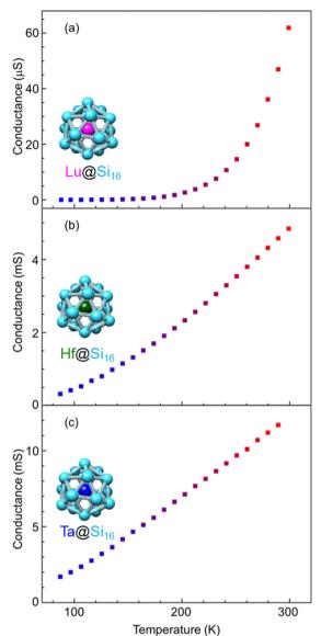
Fig. 8 Metal-atom dependence of temperature-dependent electrical conductance for different group-3, -4, and -5; (a) Lu@Si $_{16}$ , (b) Hf@Si $_{16}$ , and (c) Ta@Si $_{16}$  assembled films.
