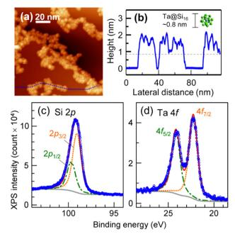
Fig. 2 Characterization of Ta@Si<sub>16</sub> deposited on a HOPG surface. (a) An STM image with (b) the height profile taken along a blue-dotted line in (a). XPS spectra for around (c) Si 2p and (d) Ta 4f core levels with the fitted results. Reproduced with permission from ref. 105. Copyright 2015 American Chemical Society
