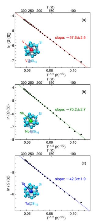
Fig. 7 Temperature dependent electrical conductance of  $M^V@Si_{16}$  $(M^V = (a) V, (b) Nb, and (c) Ta)$  assembled films based on ES-VRH. Logarithm of conductance (ln  $\it G$ ) versus  $\it T^{-1/2}$  for  $\it M^V @ Si_{16}$  films is plotted at 87-300 K, and the slope values are shown in each. Reproduced with permission from ref. 33. Copyright 2021 American Chemical Society.
