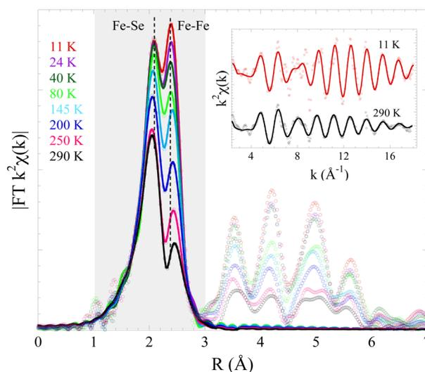
Fig. 3 Fourier transform magnitudes of the EXAFS oscillations measured on  $(\text{Li}_{1-x}\text{Fe}_x)\text{OHFeSe}$  (weighted by  $k^2$ ) at several temperatures (symbols) together with the five-shell model fits (solid lines). The fit interval is shown by the shaded area. The inset shows EXAFS oscillations (not filtered) with the model fits as above for two representative temperatures.
