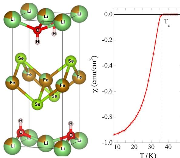
Fig. 1 Crystal unit cell of (Li<sub>1-x</sub>Fe<sub>x</sub>)OHFeSe prepared using Vesta<sup>46</sup> is displayed (left) together with the magnetic susceptibility curve showing (right) the superconducting transition temperature ( $T_c$ ). In the structural unit cell the partial substitutions of Li/Fe sites are indicated by different colors.
