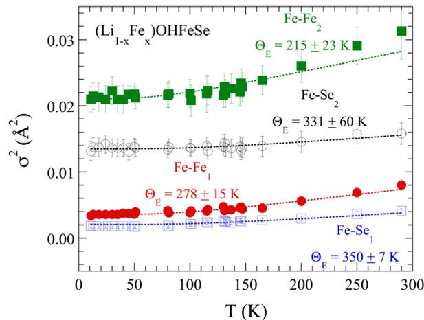
Fig. 7 Temperature dependence of the mean square relative displacements of near-neighbor bond lengths for the  $(\text{Li}_{1-x}\text{Fe}_x)\text{OHFeSe}$  system; local Fe–Se (open symbols) and Fe–Fe (filled symbols). The dotted lines represent the Einstein model fits.
