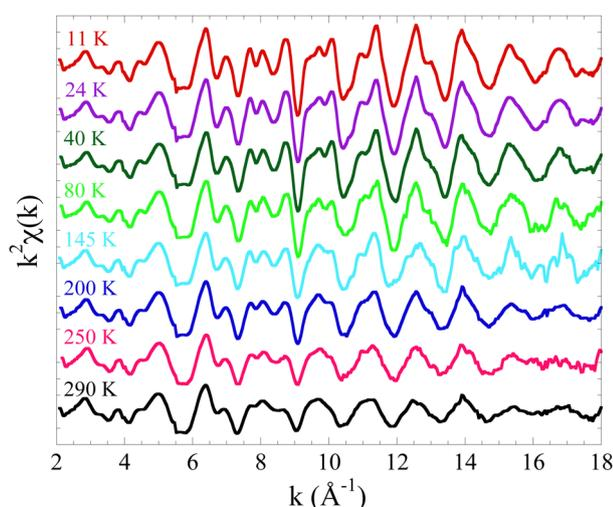
Fig. 2 Temperature evolution of EXAFS oscillations (weighted by  $k^2$ ) extracted from the Fe K-edge X-ray absorption spectra of  $(\text{Li}_{1-x}\text{Fe}_x)\text{OHFeSe}$  single crystals. The EXAFS spectra are shifted vertically for a better visualization.
