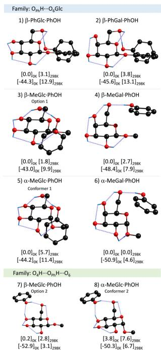
**Fig. 3** Assigned structures of PhOH aggregates with β-PhGlc, β-PhGal, β-MeGlc, β-MeGal, α-MeGlc and α-MeGal, computed at the M06-2x/6-311++G(d,p) level. Numbers in brackets are the relative energy and the binding energy in kJ mol $^{-1}$  calculated at the specified temperatures. The rest of the computed structures may be found in the ESI.†
