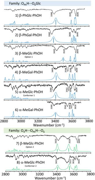
**Fig. 2** Mass-resolved IR spectra of PhOH aggregates with β-PhGlc, β-PhGal, β-MeGlc, β-MeGal,  $\alpha$ -MeGlc and  $\alpha$ -MeGal, together with the simulated spectra of the isomers to which they were assigned (in blue), built using the normal mode analysis computed at the M06-2x/6-311++G(d,p) level, and the procedure described in the Methods section.
