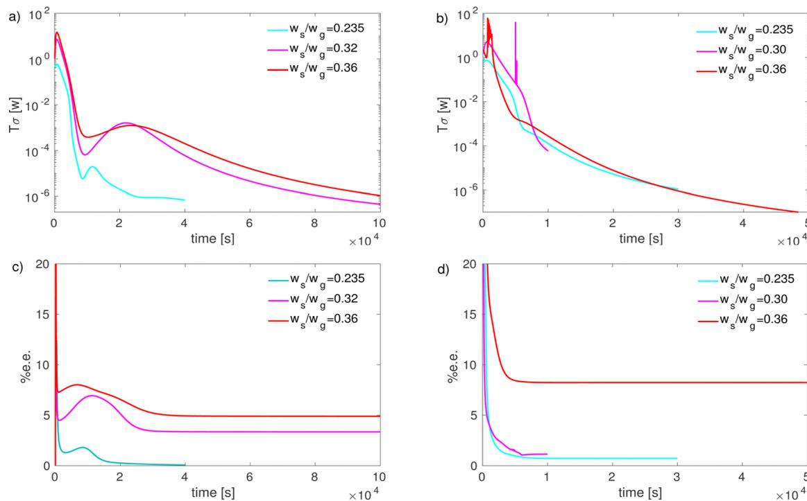
Fig. 7 Energy dissipation rate and enantiomeric excess percentage as a function of time for different values of  $w_s/w_g$ : natural cooling (a and c), and enhanced cooling (b and d).
