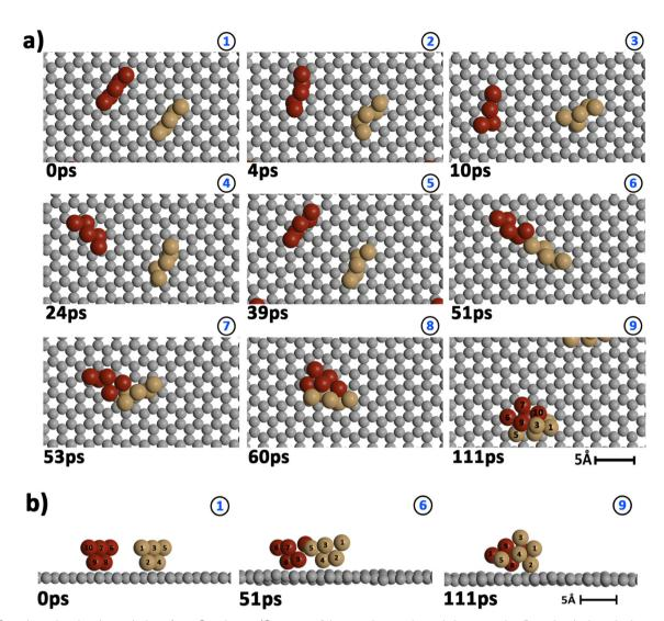
Fig. 3 Snapshots showing the evolution of two Cu<sub>5</sub> clusters (Cu atoms of the two clusters shown in brown and red) previously deposited onto a defectfree graphene surface (C atoms in gray) at a temperature of 400 K. (a) Top view; (b) side view.
