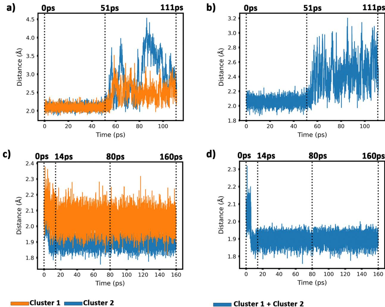
**Fig. 7** Time-dependent evolution of the minimum C–Cu distances for (a) the interaction of the two 2D–Cu<sub>5</sub> clusters with defect-free graphene; (b) the interaction of all Cu atoms with defect-free graphene; (c) the interaction of the two 2D–Cu<sub>5</sub> clusters with defected graphene; (d) the interaction of all Cu atoms with defected graphene.
