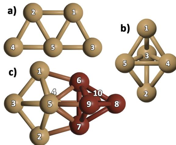
Fig. 1 Optimized structures of individual  $\text{Cu}_5$  clusters (above, a and b panels) and the  $\text{Cu}_{10}$  dimer (below, c panel) in the lowest-energy configurations. Atom numbering included. Different colors (brown and dark-red) are used for Cu atoms from the two  $3\text{D-Cu}_5$  structures composing the  $\text{Cu}_{10}$  dimer.
