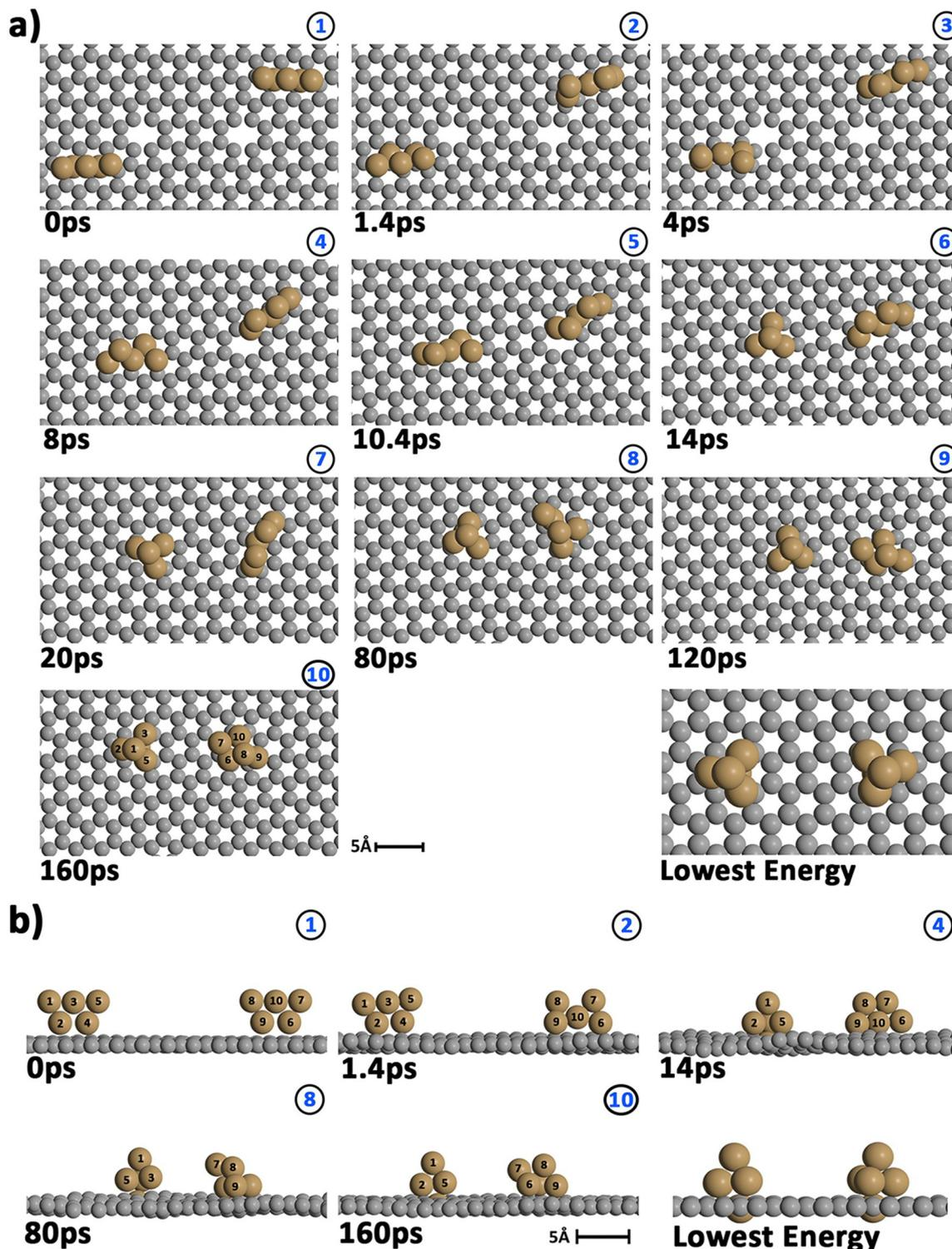
Fig. 4 Snapshots showing the evolution of two  $\text{Cu}_5$  clusters (Cu atoms in brown) previously deposited onto a graphene sheet containing two carbon vacancies (C atoms in gray) at a temperature of 400 K. (a) Top view; (b) side view.
