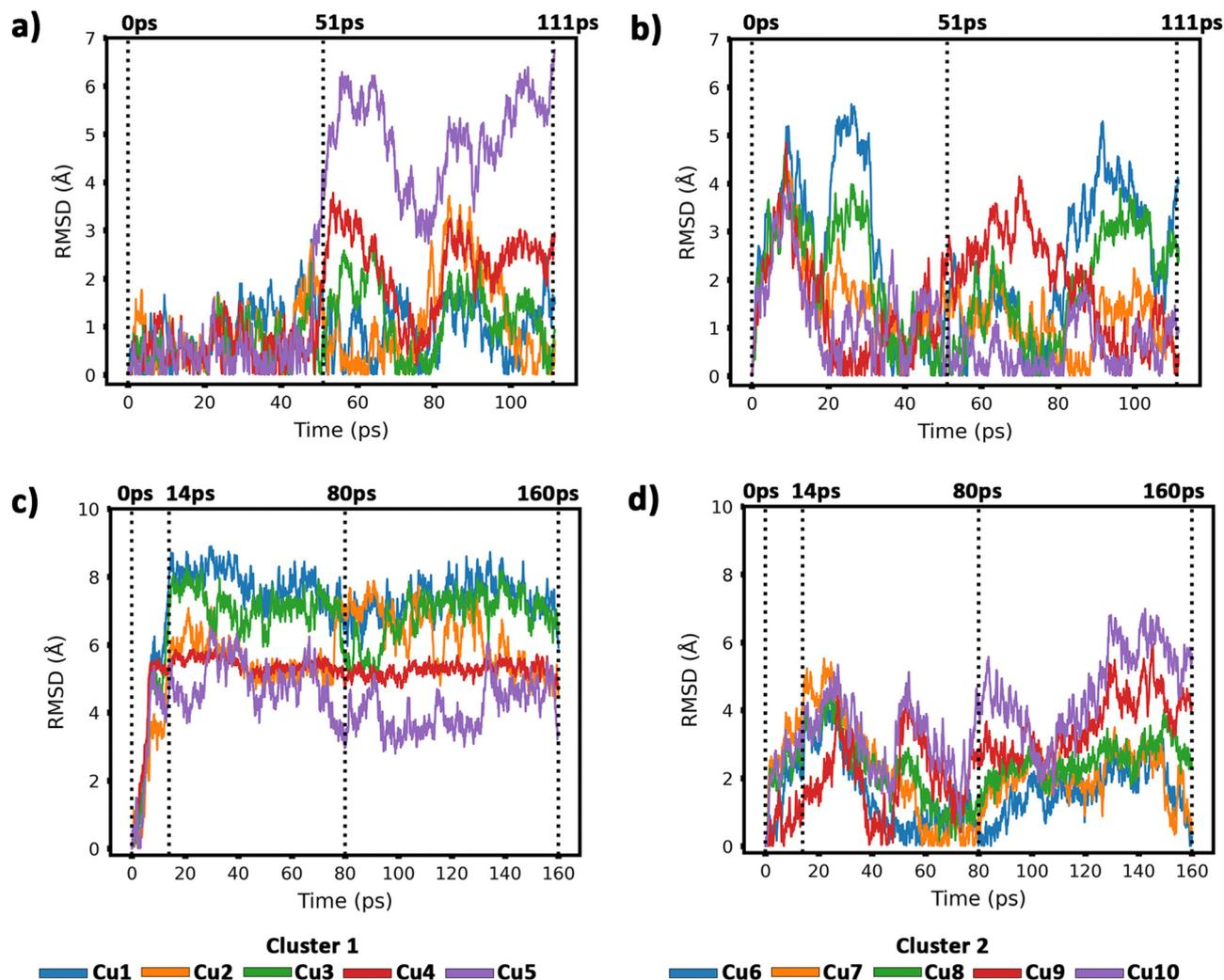
Fig. 6 Root-mean-square deviations (RMSDs) of copper atomic positions for the two  $\text{Cu}_5$  clusters supported on defect-free graphene [panels (a) and (b)] and supported on defected graphene [panels (c) and (d)] (see also Fig. 4 and 5).
