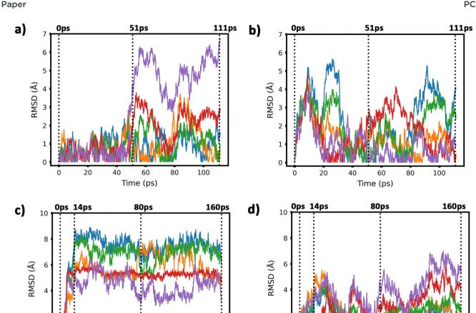
Fig. 6 Root-mean-square deviations (RMSDs) of copper atomic positions for the two Cu<sub>5</sub> clusters supported on defect-free graphene [panels (a) and (b)] and supported on defected graphene [panels (c) and (d)] (see also Fig. 4 and 5).
