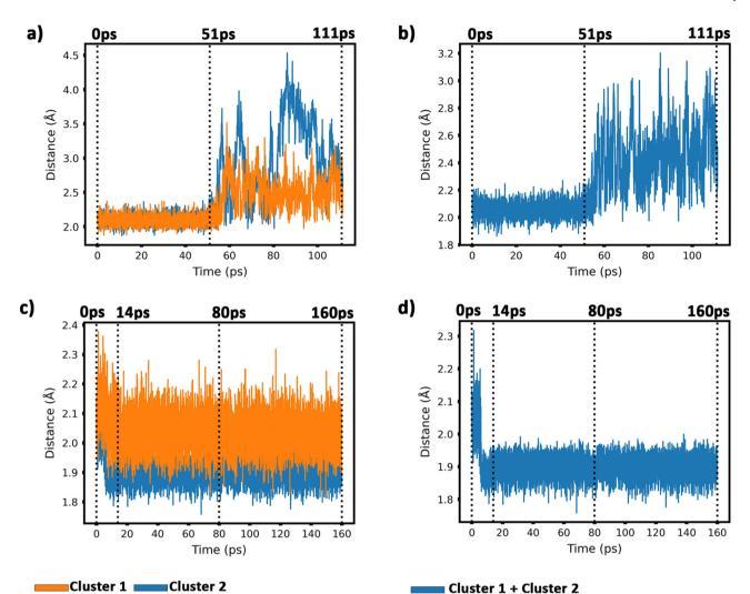
Fig. 7 Time-dependent evolution of the minimum C-Cu distances for (a) the interaction of the two  $2D-Cu_5$  clusters with defect-free graphene; (b) the interaction of all Cu atoms with defect-free graphene; (c) the interaction of the two  $2D-Cu_5$  clusters with defected graphene; (d) the interaction of all Cu atoms with defected graphene.
