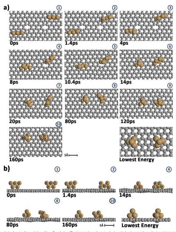
Fig. 4 Snapshots showing the evolution of two Cu<sub>5</sub> clusters (Cu atoms in brown) previously deposited onto a graphene sheet containing two carbon vacancies (C atoms in gray) at a temperature of 400 K. (a) Top view; (b) side view.
