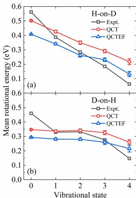
Fig. 6 Comparison of the mean rotational energy as a function of vibrational state for the H-on-D (a) and D-on-H (b) collisions obtained from QCT(EF) and experiments. The experimental data are taken from ref. 13 at  $E_{in} = 0.07$  eV and  $\theta_{in} = 10^\circ$ .
