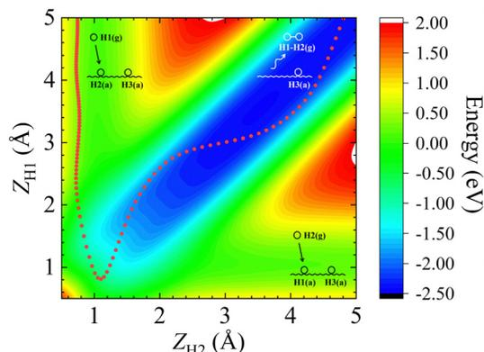
**Fig. 2** Two-dimensional energy contour plot for showing the ER and exchange channels (corresponding structures illustrated by insets) as a function of  $Z_{H1}$  (distance between the surface and H1) and  $Z_{H2}$  (distance between the surface and H2). A representative ER trajectory is projected onto this contour plot by red dots. The energy zero is the same as that shown in Fig. 1.
