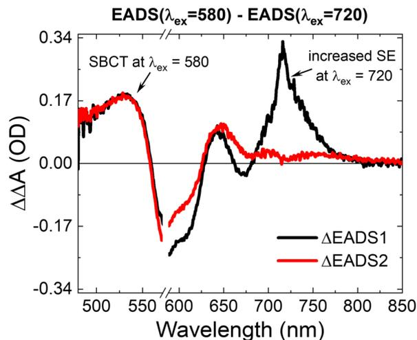
Fig. 6 Calculated difference spectrum between EADS fits for  $\alpha$ -CuPc thin film excited at  $\lambda_{\text{ex}} = 580$  nm and  $\lambda_{\text{ex}} = 720$  nm shows features consistent with symmetry-breaking charge-transfer at  $\lambda_{\text{ex}} = 580$  nm and increased relative stimulated emission at  $\lambda_{\text{ex}} = 720$  nm.
