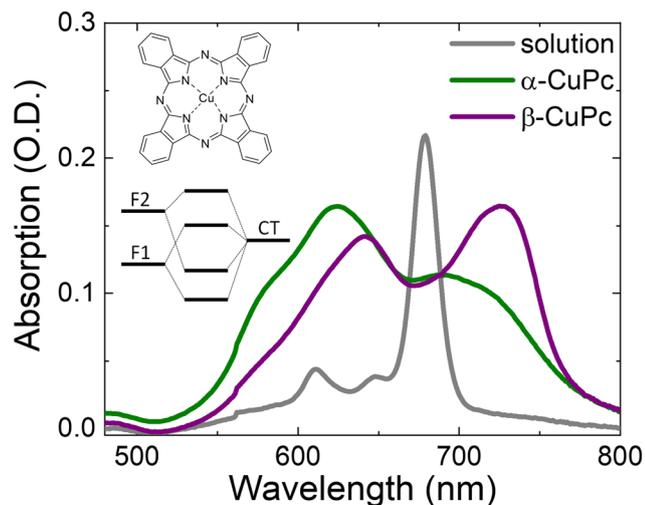
Fig. 1 Steady-state absorption of CuPc in 1-chloronaphthalene solution and in thin films with  $\alpha$ - and  $\beta$ -phase stacking morphologies in the spectral range of the Q-band absorption. The film samples exhibit different absorption peak positions and relative intensities due to changes in intermolecular couplings.
