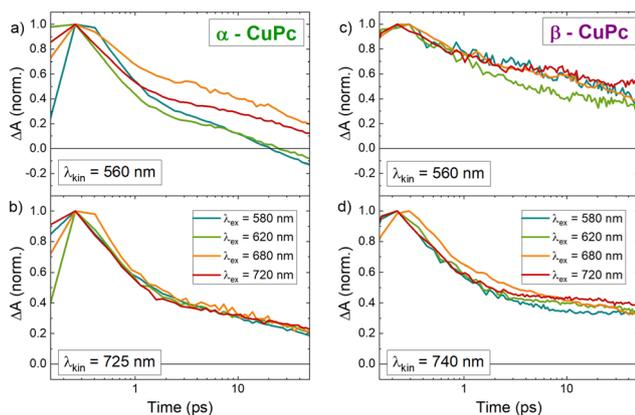
Fig. 5 Transient kinetics for (a and b)  $\alpha$ -CuPc and (c and d)  $\beta$ -CuPc thin films show that at 560 nm, the  $\alpha$ -CuPc decay dynamics vary with excitation wavelength. The decay dynamics of  $\beta$ -CuPc at 560 nm do not exhibit any such dependence. Furthermore, the kinetics associated with the SE quenching at 725 and 740 nm do not depend on excitation wavelength in either sample. Data truncated to the first 50 ps.
