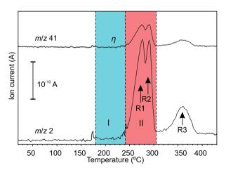
Fig. 1 Mass-spectrometric signals with increasing temperature; region I corresponds to the initial stage after melting (T = 180-240 °C); region II corresponds to the main stage at which H2 emission occurs via reactions (R1) and (R2) (T = 240-305 °C)
