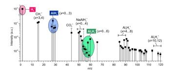
Fig. 2 The mass spectrum of gases emitted during rubbing of NaAlH<sub>4</sub>. Hydrogen is the dominating species exceeding other components by 3 to
