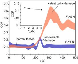
Fig. 10 The time series of coefficient of friction at various normal loads. Two regimes can be seen: normal friction and catastrophic damage. The inset shows the effect of the normal load on the normal COF.
