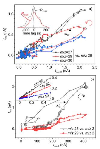
Fig. 4 Correlation analysis of mass-spectrometer signals: (a) m/z 27, 29 and 30 vs. m/z 28; (b) m/z 28 and 29 vs. m/z 2. The inset in (a) shows crosscorrelation graphs for 27-28 and 29-27 signals. The inset in (b) shows the signals with m/z 50, 52 and 53 vs. m/z 51. The dashed arrows show the directions of the evolution of the signals with time in the corresponding
