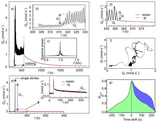
Fig. 7 (a) Time series of H<sub>2</sub> emission rate measured using an ion gauge; (b and d) the enlarged portions of the emission rate time series; (c) spectral power density of the emission rate oscillations; (e) gas emission response to a single rubbing stroke; (f) cross-dependencies between  $Q_1$  and  $Q_2$ ; (g) cross-correlation function of  $Q_2$  concerning  $Q_1$ , the blue area denotes the portion of the graph, which deviates from symmetry
