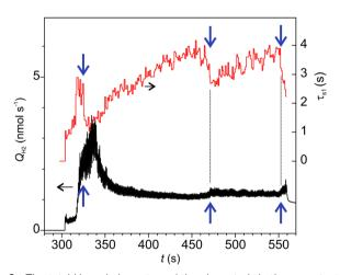
Fig. 8 The total H<sub>2</sub> emission rate and the characteristic time constant of transient decays during time lags between consecutive rubbing cycles. The arrows show the occasional events when the emission rate suddenly increased and the time constant decreased.
