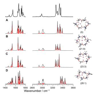
Fig. 4 Calculated IR spectra of conformers A-D for Li<sup>+</sup>VM with the experimental IRPD spectrum. Parentheses indicate the relative Gibbs free energy for each conformer at 298 K.
