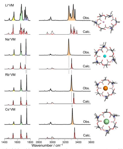
Fig. 2 IRPD spectra of Li<sup>+</sup>, Na<sup>+</sup>, Rb<sup>+</sup>, and Cs<sup>+</sup>VM complexes. The calculated IR spectrum of the most stable conformer at 298 K is shown with its molecular structure for each IRPD spectrum. The black solid curves in the calculated spectra are made by convolution of stick red lines. Color codes: gray = C, blue = N, red = O, white = H, pink = Li, cyan = Na, orange = Rb, light green = Cs. The IRPD spectrum of K<sup>+</sup> complex is shown in Fig. S3 in ESI.†
