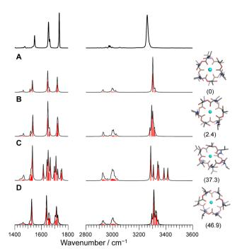
Fig. 3 Calculated IR spectra of conformers A–D for Na<sup>+</sup>VM with the experimental IRPD spectrum. Parentheses indicate the relative Gibbs free energy for each conformer at 298 K.
