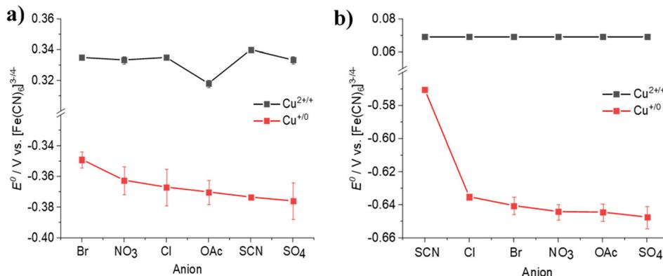
Fig. 2 Redox potentials obtained from the different copper salts (each  $0.02 \text{ mol dm}^{-3}$ ) in: (a) EG:ChCl, and (b)  $\text{CaCl}_2 \cdot 6\text{H}_2\text{O}:\text{EG}$ , presented as a function of salt anion. All potentials were corrected for small changes in concentration and temperature using the Nernst equation, and referenced to the  $[\text{Fe}(\text{CN})_6]^{3-/4-}$  couple.
