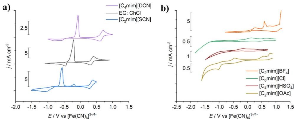
Fig. 5 Cyclic voltammograms of copper salts in EG:ChCl and six ILs at a Pt-disc working electrode, with a scan rate of  $10 \text{ mV s}^{-1}$ . The current density was normalised to remove any current effects due to the different solvent viscosity values. CVs are referenced to the  $[\text{Fe}(\text{CN})_6]^{3-/4-}$  redox couple. Presented data is the first scan.
