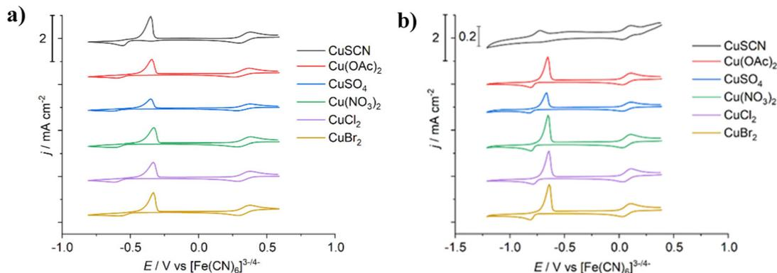
Fig. 1 Cyclic voltammograms of the different copper salts (each 0.02 mol dm<sup>-3</sup>) in: (a) EG:ChCl, and (b) CaCl<sub>2</sub>·6H<sub>2</sub>O:EG at a 0.5 mm diameter Pt-disc, referenced to the [Fe(CN)<sub>6</sub>]<sup>3-/4-</sup> redox couple, with a scan rate of 20 mV s<sup>-1</sup>. Temperature = 20 °C. CVs offset for clarity. Presented data is the first scan. Note that CuSCN in CaCl<sub>2</sub>·6H<sub>2</sub>O:EG is on a different scale to the other systems.
