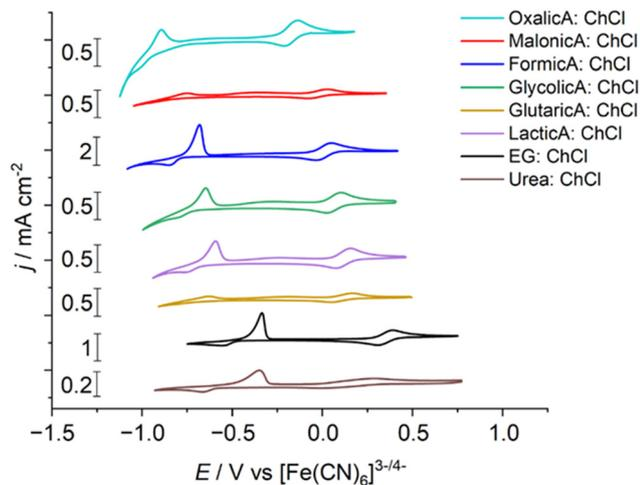
Fig. 7 Cyclic voltammograms of copper(II) chloride ( $0.02 \text{ mol dm}^{-3}$ ) in the 8 different DESs at a  $0.5 \text{ mm}$  diameter Pt-disc, referenced to the  $[\text{Fe}(\text{CN})_6]^{3-/4-}$  redox couple, with a scan rate of  $20 \text{ mV s}^{-1}$ . Temperature =  $20 \text{ }^\circ\text{C}$ . CVs are offset for clarity, with EG:ChCl included as a comparison. Presented data is the first scan.
