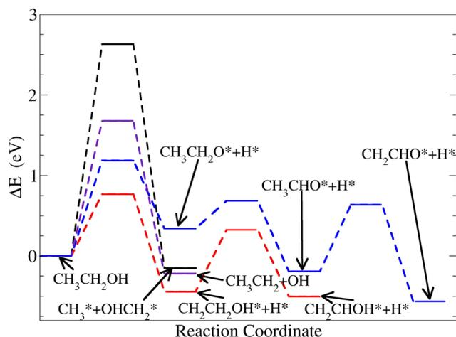
Fig. 8 Energy profiles of the four alternative reaction pathways with an adsorbed ethanol starting on Pos3 on Pt<sub>38</sub>.
