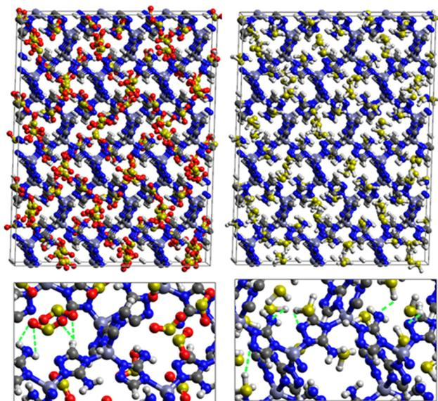
**Fig. 5** Top: GCMC adsorption sites of SO<sub>2</sub> (left) and H<sub>2</sub>S (right) molecules inside the pores of MAF-66. Bottom: Enlargement in the vicinity of SO<sub>2</sub> and H<sub>2</sub>S molecules where non-bonded interactions are also shown.
