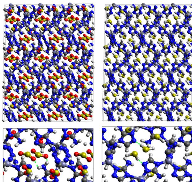
**Fig. 1** Top: DFT optimized 3D structures of SO<sub>2</sub> (left) and H<sub>2</sub>S (right) inside MAF-66. Bottom: Enlargement in the vicinity of SO<sub>2</sub> and H<sub>2</sub>S molecules where non-bonded interactions are also shown with green dashed lines.
