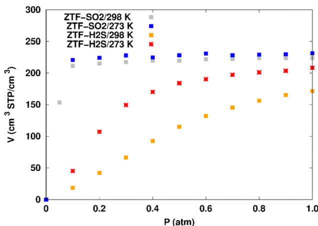
**Fig. 6** Simulated adsorption isotherms of SO<sub>2</sub> and H<sub>2</sub>S in ZTF at 273 and 298 K.
