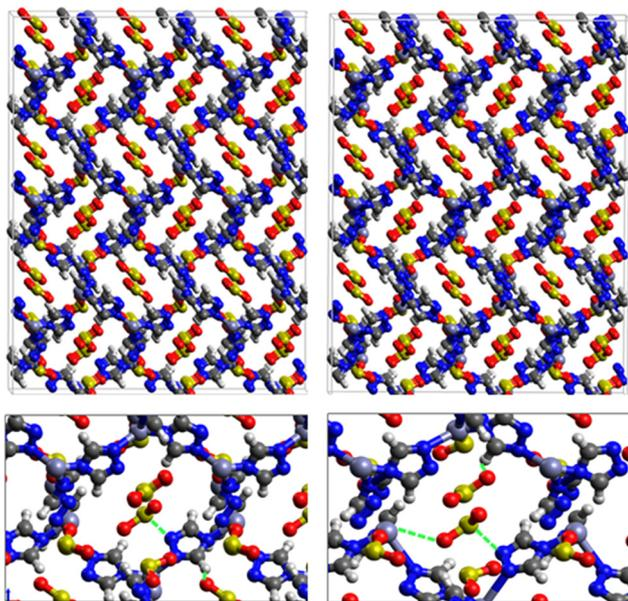
Fig. 2 Top: DFT optimized 3D structures of  $\text{SO}_2$  inside ZTF with binding energies of  $-7.48 \text{ kcal mol}^{-1}$  (left) and of  $-9.00 \text{ kcal mol}^{-1}$  (right). Bottom: Enlargement in the vicinity of  $\text{SO}_2$  molecules where non-bonded interactions are also shown with green dashed lines.
