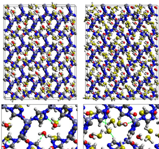
Fig. 11 Top: GCMC adsorption sites of  $\text{H}_2\text{S}$  molecules inside the pores of ZTF in the presence of  $\text{H}_2\text{O}$  near the nitrogen atom of the triazole subunits (left) or near the Zn atom (right). Bottom: Enlargements in the vicinity of  $\text{H}_2\text{S}$  and  $\text{H}_2\text{O}$  where non-bonded interactions are also highlighted.
