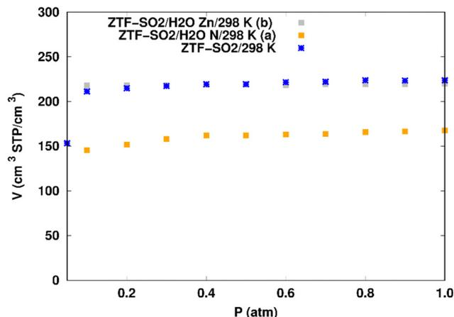
Fig. 8 Simulated adsorption isotherms of  $\text{SO}_2$  at 298 K in ZTF with and without the presence of water molecules, where  $\text{H}_2\text{O}$  is located near a nitrogen of the surface pore (in (a)) or in the vicinity of the Zn atom (in (b)).
