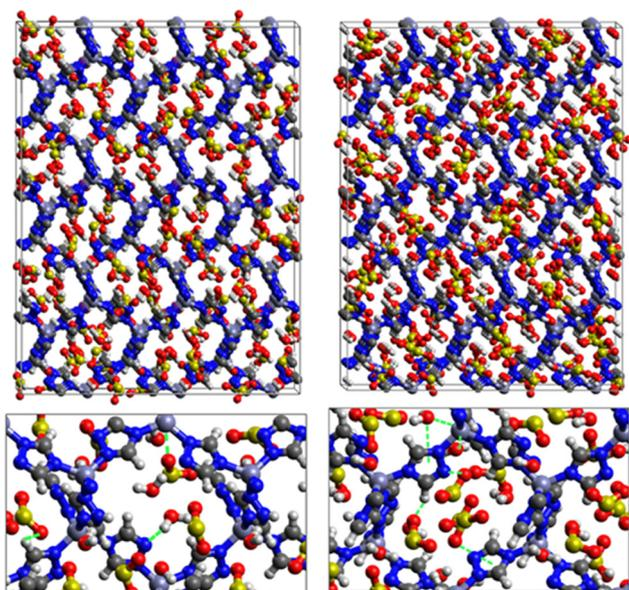
Fig. 9 Top: GCMC adsorption sites of  $\text{SO}_2$  molecules inside the pores of ZTF in the presence of  $\text{H}_2\text{O}$  near the nitrogen atom of the triazole subunits (left) or near the Zn atom (right). Bottom: Enlargement in the vicinity of  $\text{SO}_2$  and  $\text{H}_2\text{O}$  where non-bonded interactions are also highlighted.
