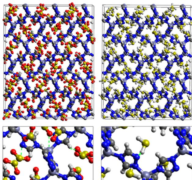
Fig. 7 Top: GCMC adsorption sites of SO<sub>2</sub> (left) and H<sub>2</sub>S (right) molecules inside the pores of ZTF. Bottom: Enlargement in the vicinity of SO<sub>2</sub> and H<sub>2</sub>S with non-bonded interactions are also presented.
