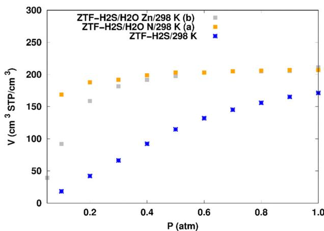
Fig. 10 Simulated adsorption isotherms of  $\text{H}_2\text{S}$  at 298 K in ZTF with and without the presence of water molecules, where  $\text{H}_2\text{O}$  is located near nitrogen (in (a)) or in the vicinity of the Zn atom (in (b)).
