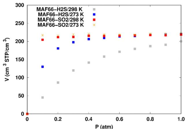
**Fig. 4** Simulated adsorption isotherms of SO<sub>2</sub> and H<sub>2</sub>S in MAF-66 at 273 and 298 K.
