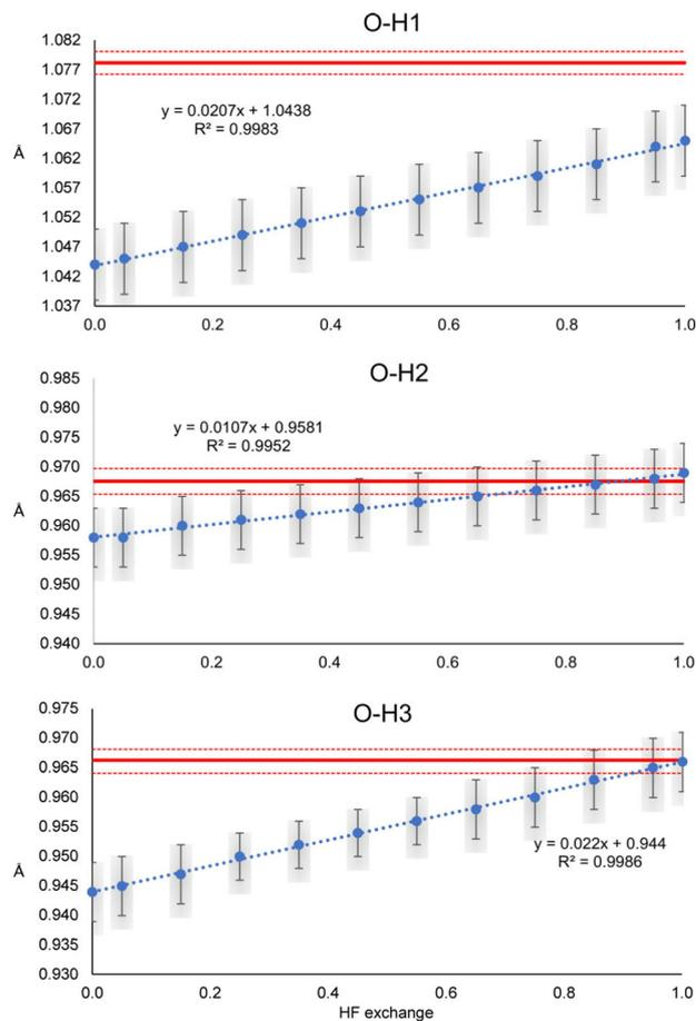
Fig. 3 O–H1, O–H2 and O–H3 distances refined with the HAR for different percentages of HF exchange with the  $PBE_x$  and the def2-TZVP basis set. The red line corresponds to the neutron diffraction value. The least-squares std errors of the HAR and neutron diffraction are shown as blue bars and red dashed lines, respectively.
