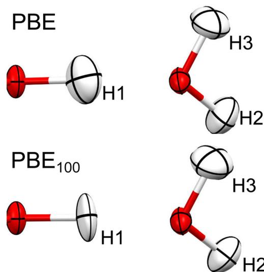
Fig. 10 Thermal ellipsoids (at 50% probability) of H1, H2 and H3 of oxalic acid obtained from HAR, using PBE and PBE<sub>100</sub>.
