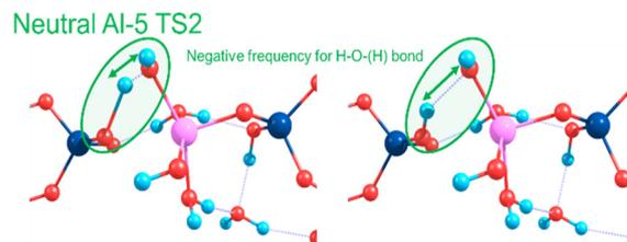
**Fig. 1** Atomic motions along the negative frequency mode during the proton transfer from Si–OH to form Al–OH<sub>2</sub> as part of the second transition state for the neutral mechanism using Al-5.
