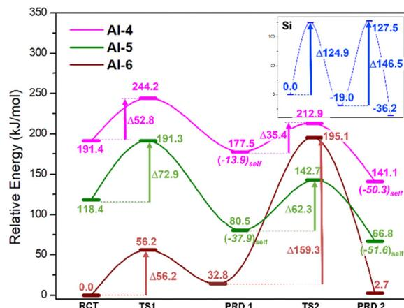
Fig. 3 Neutral mechanism: relative free energy ( $\Delta G_{\text{rel}}$ ) for differing Al-coordinations with respect to reactants: Al-IV (magenta) Al-V (green) and Al-VI (rust-red). Inset: Si-only mechanism (blue) devoid of an Al-centre. Isodesmic comparison of free energies is possible between differing Al-coordinations by adding or subtracting the energy of one water molecule, generating the relative-relative free-energies ( $\Delta\Delta G_{\text{rel}}$ ).
