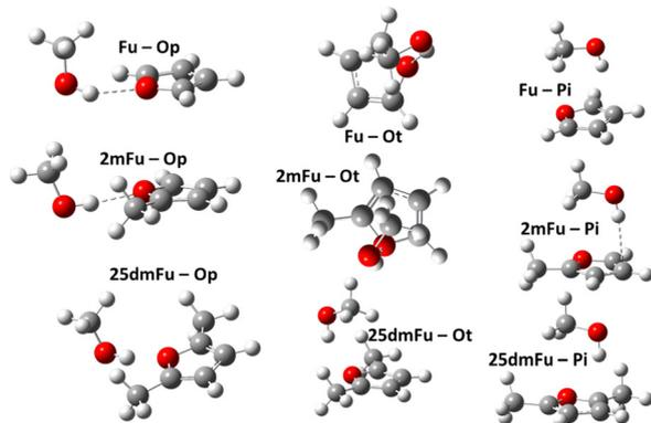
Fig. 1 Main minimum-energy structures used in this study: OH-bonded complexes of furan (Fu), 2-methylfuran (2mFu), and 2,5-dimethylfuran (25dmFu) with methanol in plane (p) and top (t) configuration and their  $\pi$ -bonded counterparts.
