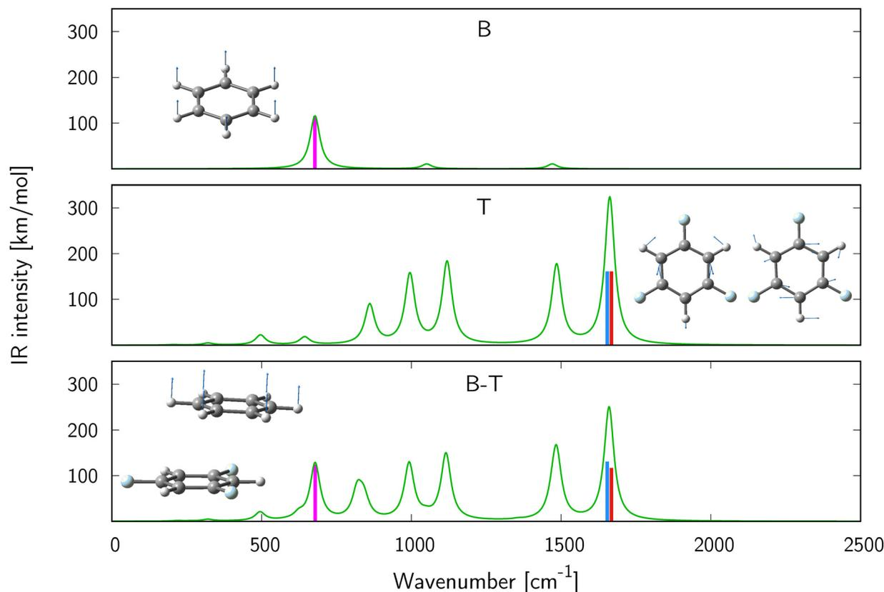
Fig. 1 Simulated IR spectra of benzene (top), 1,3,5-trifluorobenzene (middle) and their complex (bottom). Insets show atomic displacements corresponding to vibrational normal mode  $\nu_6$  of benzene (top),  $\nu_{26}$  and  $\nu_{27}$  (middle) mode of 1,3,5-trifluorobenzene, and  $\nu_{24}$  (bottom) of the complex. Bands corresponding to C–H stretching ( $>3000\text{ cm}^{-1}$ ) are not shown.
