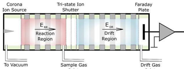
**Fig. 1** The HiKE-IMS has been described previously, but briefly, the HiKE-IMS is divided into two regions: the reaction region and the drift region.<sup>31</sup> Both sections have an electric field that can be changed independently of each other which allows for examination of the speciation of each ion based on explicit operating parameters.
