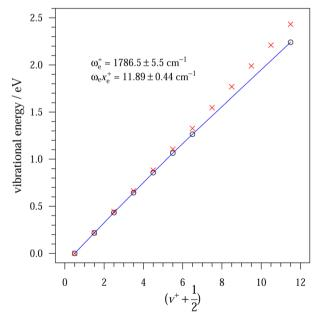
Fig. 3 Energies of the lowest vibrational levels of the electronic ground state of CF<sup>+</sup> with respect to its  $v^+ = 0$  level as a function of  $(v^+ + \frac{1}{2})$ . The red crosses represent our harmonic calculations and the black circles our measurements. The blue line corresponds to a second-order polynomial fit of our experimental values. See the text for details.
