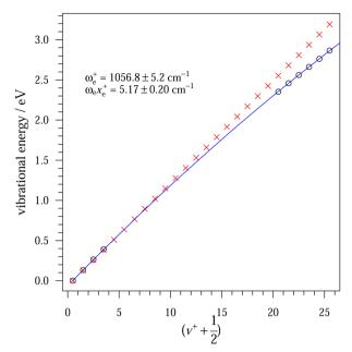
Fig. 6 Energies of the lowest vibrational levels of the electronic ground state of SiF<sup>+</sup> with respect to its  $v^+ = 0$  level as a function of  $(v^+ + \frac{1}{2})$ . The red crosses represent our harmonic calculations and the black circles our measurements. The blue line corresponds to a second-order polynomial fit of our experimental values
