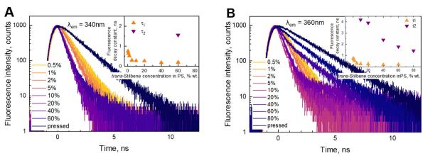
Fig. 3 Fluorescence decay kinetics of trans-stillbene in the PS matrix at 340 nm (A) and 360 nm (B) under 300 nm excitation. Dependences of the fluorescence decay constants ( $\tau_1$  and  $\tau_2$ ) on the stilbene concentration in the PS matrix are presented in the insets.
