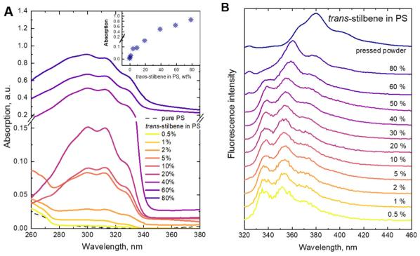
Fig. 1 (A) Normalized absorption spectra of trans-stillbene in the PS matrix; in the inset, the dependence of the absorption at 312 nm on the transstilbene concentration in the PS matrix is shown. (B) Normalized fluorescence spectra of trans-stilbene in the PS matrix under 300 nm excitation.
