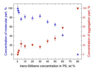
Fig. 6 Molecular (blue triangles) and aggregate (red triangles) parts of fluorescence trans-stilbene dependence on concentration in the PS matrix. The points present amplitudes in decomposition of Fig. 4A
