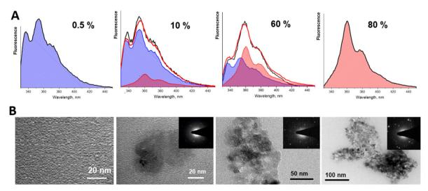
Fig. 4 (A) The normalized fluorescence spectra obtained (black line) and reconstructed (red line) at different concentrations of trans-stilbene in the PS matrix. Fluorescence spectra filled in blue demonstrate a molecular part of trans-stilbene fluorescence and those of aggregates (or nanocrystals) in pink. Note that there is still a small contribution of molecular fluorescence at 80% concentration. Amplitudes of decomposition are presented in Fig. 6. (B). TEM images of the same films.
