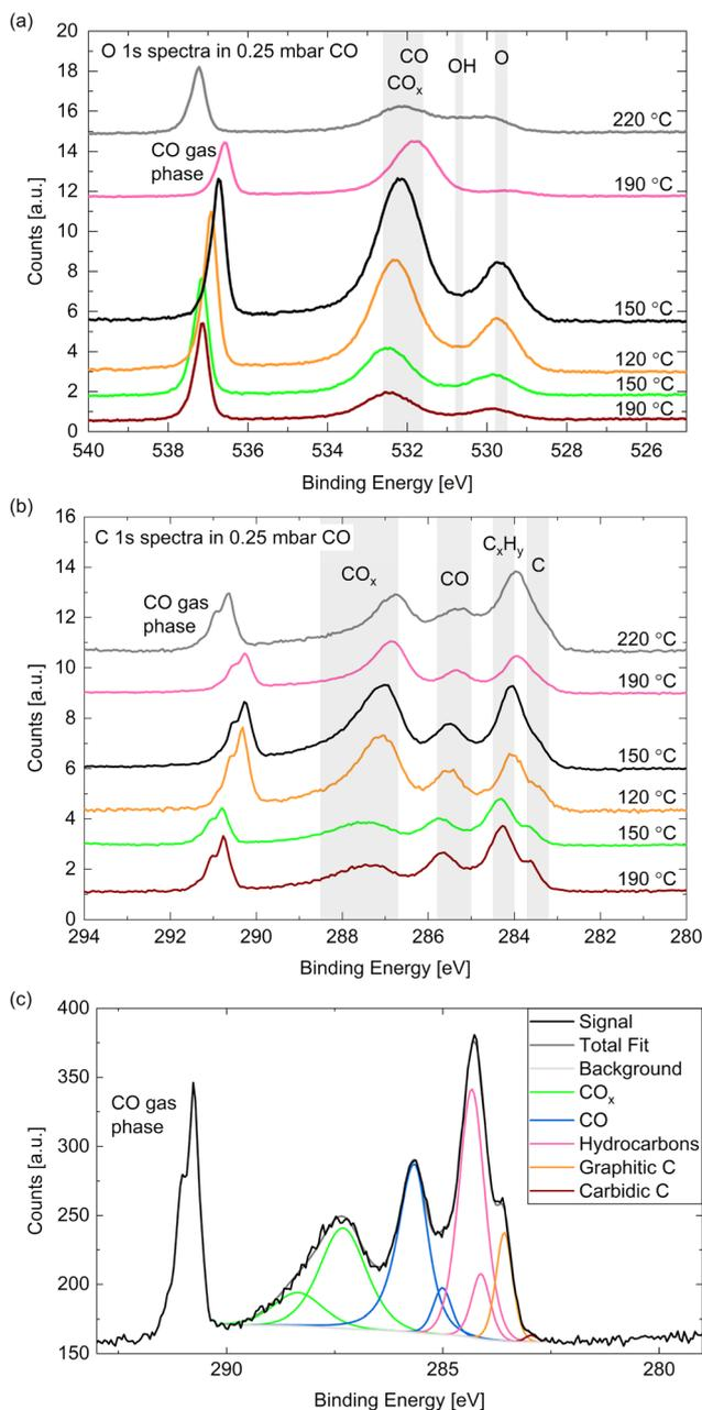
**Fig. 5** (a) O 1s and (b) C 1s spectra measured on Co(0001) in 0.25 mbar CO at different temperatures. For quantitative comparison the spectra are calibrated to the Co 2p peak area as explained above. (c) C 1s area measured on Co(0001) in 0.25 mbar CO at 190 °C surface temperature showing the peaks necessary for a satisfactory fit.
