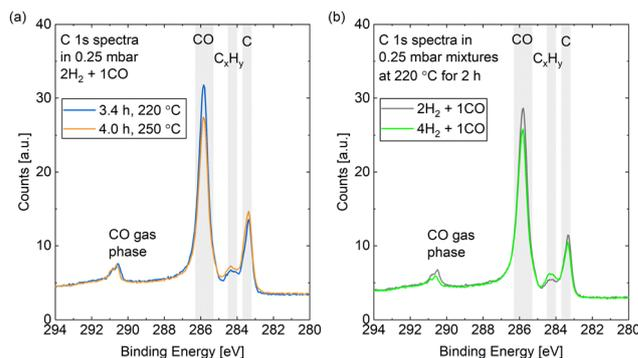
**Fig. 9** C 1s spectra measured (a) in 0.25 mbar  $2\text{H}_2 + 1\text{CO}$  comparing a measurement at  $220^\circ\text{C}$  to a subsequent one at  $250^\circ\text{C}$  and (b) at  $220^\circ\text{C}$  comparing a measurement in 0.25 mbar  $2\text{H}_2 + 1\text{CO}$  to one in 0.25 mbar  $4\text{H}_2 + 1\text{CO}$ .
