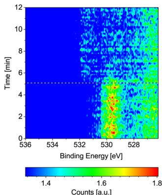
Fig. 4 O 1s spectra measured on Co(0001) over time while introducing CO at 220 °C. The black and white reference line marks the start of the flow of 1.9 ml min<sup>-1</sup> CO.
