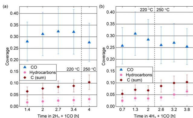
**Fig. 10** Estimated coverages of CO, hydrocarbons, and carbon (sum of the graphitic and the carbidic carbon) in (a) 0.25 mbar  $2\text{H}_2 + 1\text{CO}$  and (b) 0.25 mbar  $4\text{H}_2 + 1\text{CO}$  over time at two different temperatures. Error bars indicate the estimated accuracy of the absolute coverage values due to the calibration method while relative comparisons of the different measurements are expected to be more reliable (see Methods section).
