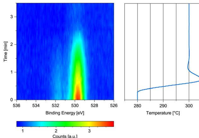
Fig. 3 O 1s spectrum measured on previously oxidized Co(0001) in 0.25 mbar dried H<sub>2</sub> while increasing the temperature from 280 °C to 300 °C with the corresponding temperature graph.
