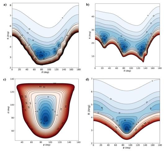
Fig. 7 2D contour plots of the 3D-PES of benzonitrile—He cluster. In (a)  $\phi = 90^{\circ}$ ; in (b)  $\phi = 0^{\circ}$ ; in (c) R = 3.15 Å; and in (d)  $\theta = 77^{\circ}$ . Energies are in cm<sup>-1</sup>.
