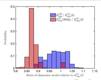
Fig. 5 The distribution of relative differences in  $E_{\text{disp}}^{(20)}$  and  $E_{\text{disp}}^{(2)}(\text{SDQ})$ dispersions with respect to the full  $E_{\text{disp}}^{(2)}(2)$  dispersion based on 330 geometries (various orientations and distances) selected for interaction energies smaller than 100 cm<sup>-1</sup>
