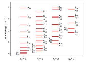
Fig. 8 The lowest 46 rotational levels of benzonitrile up to  $j_{k_a,k_c} = 9_{09}$  for rotational energy  $E_{\rm rot} \leq 5~{\rm cm}^{-1}$  with a cutoff for  $k_a$  values at  $k_a \leq 3$ . The energies of these levels were derived using a model Hamiltonian and the ground state experimental rotational and distortional constants as determined by Wlodarczak et al.74
