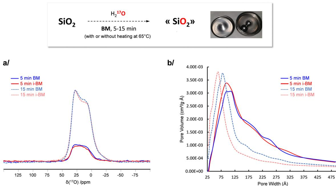
Fig. 4 Influence of i-BM on the isotopic labeling of fumed silica. (a)  $^{17}\text{O}$  MAS NMR spectra, and (b) comparison of the pore size distribution (as determined from  $\text{N}_2$  adsorption measurements, using the Barrett, Joyner et Halenda – BJH – model, as in our previous study on the  $^{17}\text{O}$ -labeling of silica),<sup>52</sup> for phases prepared after 5 and 15 minutes milling, with (red) or without (blue) i-BM.
