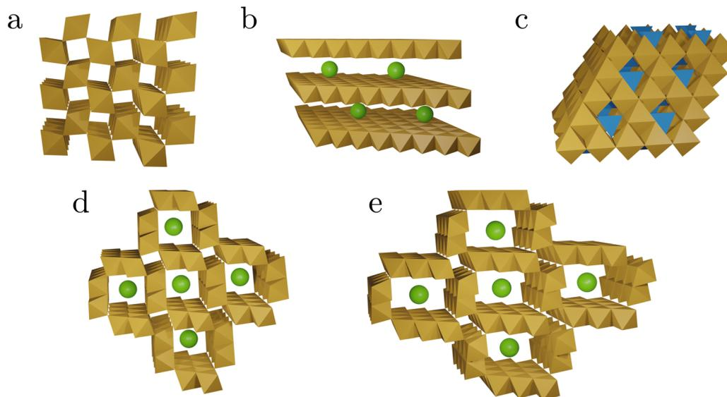
Fig. 2 Schematic representations of the tunnel and layer structures in  $\text{MnO}_x$  discussed in this work. The structures shown consist of  $\text{MnO}_6$  octahedra (brown),  $\text{MnO}_4$  tetrahedra (blue), and spheres representing other cations or water (green). Structural details are listed in Table 1. Pyrolusite,  $\beta$ - $\text{MnO}_2$  (a), birnessite  $\delta$ - $\text{MnO}_2$  (b), spinel structure (c), hollandite  $\alpha$ - $\text{MnO}_2$  (d), and romanèchite (e).
