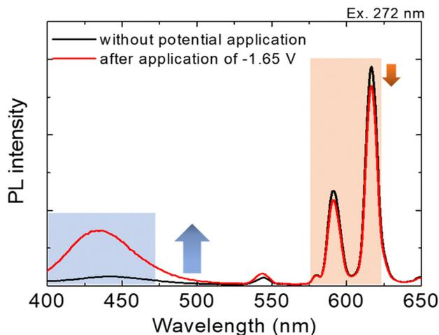
Fig. 2 Emission spectra of the  $\text{Eu}(\text{NO}_3)_3 \cdot 6\text{H}_2\text{O}$  solution in a three-electrode electrochemical cell with/without an applied reduction potential ( $-1.65 \text{ V}$ ). Excitation wavelength =  $272 \text{ nm}$ .
