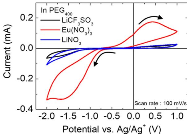
Fig. 1 Cyclic voltammograms of  $\text{Eu}(\text{NO}_3)_3 \cdot 6\text{H}_2\text{O}$  or  $\text{LiNO}_3$  in  $\text{PEG}_{400}$ . ( $[\text{LiCF}_3\text{SO}_3] = 500 \text{ mM}$ ,  $[\text{Eu}(\text{NO}_3)_3 \cdot 6\text{H}_2\text{O}] = 10 \text{ mM}$ ,  $[\text{LiNO}_3] = 60 \text{ mM}$ ).
