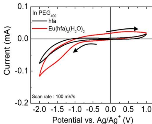
Fig. 3 Cyclic voltammograms of  $\text{Eu}(\text{hfa})_3(\text{H}_2\text{O})_2$  or hfa in  $\text{PEG}_{400}$ . ( $[\text{LiCF}_3\text{SO}_3] = 500 \text{ mM}$ ,  $[\text{Eu}(\text{hfa})_3(\text{H}_2\text{O})_2] = 10 \text{ mM}$ ,  $[\text{hfa}] = 30 \text{ mM}$ ).
