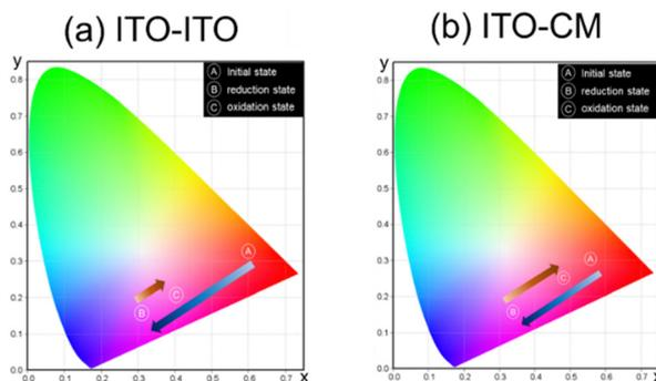
Fig. 9 The CIE chromaticity diagram of the  $\text{Eu}(\text{hfa})_3(\text{H}_2\text{O})_2$  solution in  $\text{PEG}_{400}$  using a two-electrode cell ((a) ITO-ITO or (b) ITO-CM) before and after the application of reducing and oxidizing voltages.
