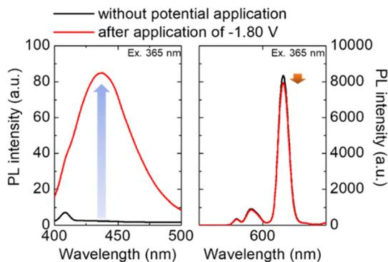
Fig. 4 Emission spectra of the  $\text{Eu}(\text{hfa})_3(\text{H}_2\text{O})_2$  solution in a three-electrode electrochemical cell with/without an applied reduction potential ( $-1.80$  V). Excitation wavelength =  $365$  nm.
