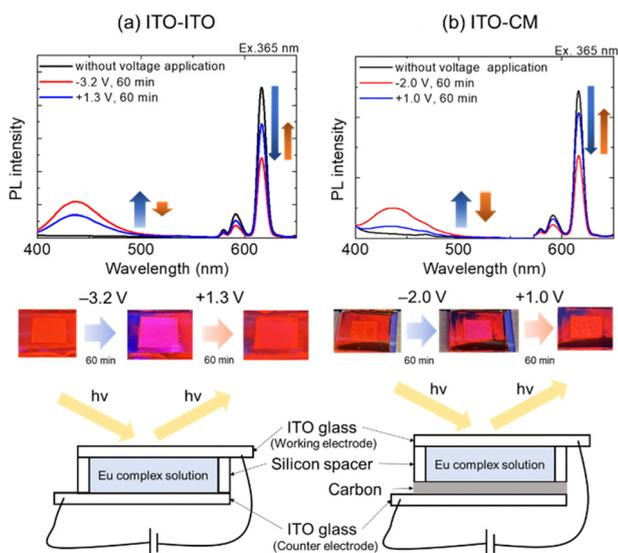
Fig. 8 Emission spectra of the  $\text{Eu}(\text{hfa})_3(\text{H}_2\text{O})_2$  solution in  $\text{PEG}_{400}$  using a two-electrode cell (a) ITO-ITO or (b) ITO-CM before and after the application of reducing and oxidizing voltages.
