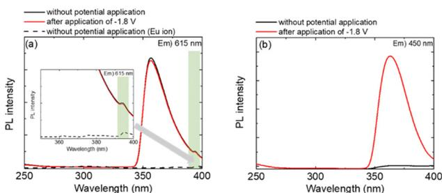
Fig. 5 Excitation spectra of the  $\text{Eu}(\text{hfa})_3(\text{H}_2\text{O})_2$  solution before and after the application of a reduction voltage. ((a) excitation wavelength =  $615$  nm), (b) excitation wavelength =  $450$  nm).
