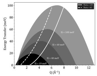
Fig. 1 Domains in the  $(Q, \omega)$  space probed by PANTHER at different incident energies ( $E_i$ ) and by the two TOSCA detector banks at  $45^{\circ}$  and 135°. For visualisation only energies up to 100 meV, in the positive energy transfer region, were plotted
