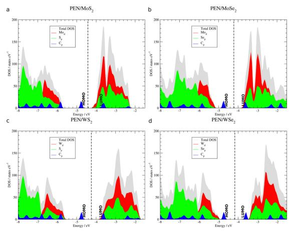
Fig. 2 Total and partial density of states (DOS) of (a) PEN/MoS<sub>2</sub>, (b) PEN/MoSe<sub>2</sub>, (c) PEN/WS<sub>2</sub> and (d) PEN/WSe<sub>2</sub> heterostructures. The Fermi level of the heterostructure is indicated by a vertical dashed line. HOMO and LUMO of pentacene are highlighted in each plot.
