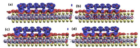
Fig. 3 Charge density difference between the heterostructures ((a) PEN/MoS<sub>2</sub>, (b) PEN/MoSe<sub>2</sub>, (c) PEN/WS<sub>2</sub> and (d) PEN/WSe<sub>3</sub>) and the isolated systems. Regions in blue and red represent depletion and accumulation of charge, respectively. Figure prepared using the XCrySDen software, 45 with isovalues in the range of -0.0001 (blue) and +0.0001 (red) e bohr<sup>-3</sup>.
