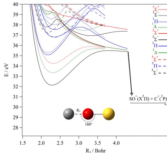
Fig. 6 MRCI/aug-cc-pV(Q+d)Z potential energy curves of the lowest electronic states of  $\text{COS}^{2+}$  along the CO coordinates ( $R_1$ ) for collinear configurations. The SO distance is set to 3.172 Bohr, *i.e.* its equilibrium value in  $\text{COS}^{2+}(\text{X}^3\Sigma^-)$ . The reference energy is that of  $\text{OCS}(\text{X}^1\Sigma^+)$  at equilibrium. Adapted from Fig. S4 (ESI<sup>†</sup>).
