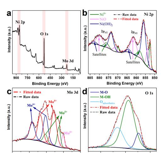
(a) XPS survey spectrum; (b) core level spectra of Ni 2p, (c) Mo 3d, and (d) O 1s for the NiMo 20 kW@100 mm sample after Al leaching.
