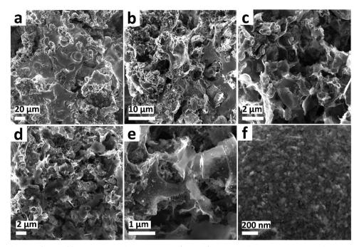
Fig. 8 SEM images of NiMo 16 kW@100 mm coating after Al leaching: (a and b) low magnification micrographs of the coating, and (c-f) higher magnification images showing the nanostructured features of the coating.
