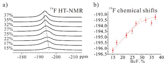
Fig. 1  $^{19}\text{F}$  HT-NMR spectra and chemical shift evolution of LiF-BeF<sub>2</sub> molten salts with different BeF<sub>2</sub> concentrations.
