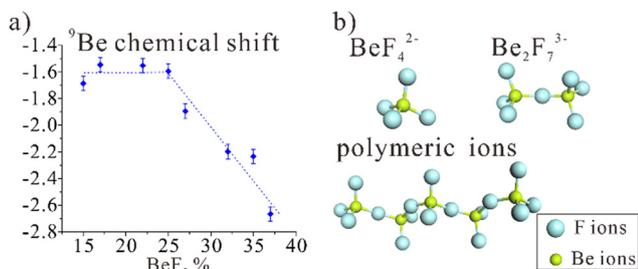
Fig. 2 (a)  $^9\text{Be}$  HT-NMR chemical shift evolution of LiF-BeF<sub>2</sub> molten salts with different BeF<sub>2</sub> concentrations. (b) Ionic structure of the BeF<sub>4</sub><sup>2-</sup> ion and the Be-F polymeric ions.
