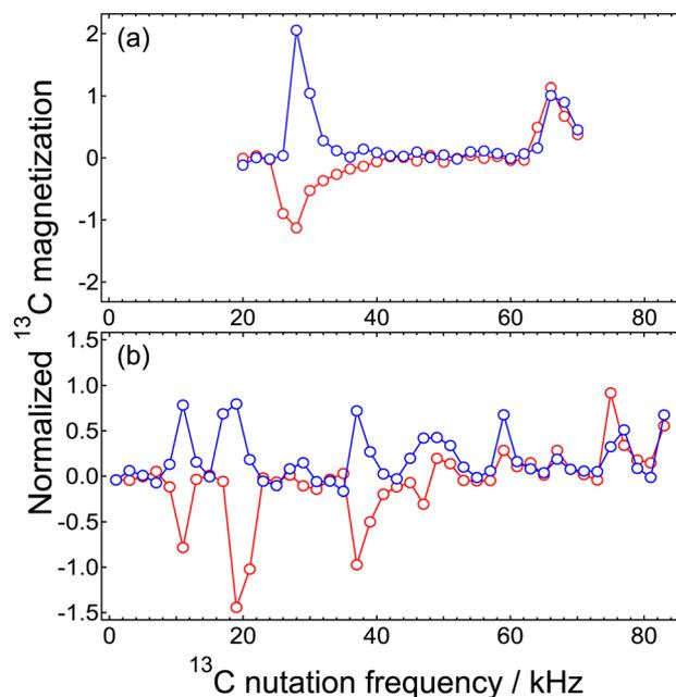
Fig. 3  $^1\text{H}$ – $^{13}\text{C}$  Hartmann–Hahn matching profiles of DONUT CP measured for adamantane in a magnetic field of 7 T under (a) the static condition and (b) MAS at 9 kHz. Red and blue circles represent the  $\omega_{1S}$  dependence obtained with ( $\omega_{11}/2\pi$ ,  $\omega_{21}/2\pi$ ) of (50 kHz, 20 kHz) and (20 kHz, 50 kHz), respectively. The contact time was 7 ms.
