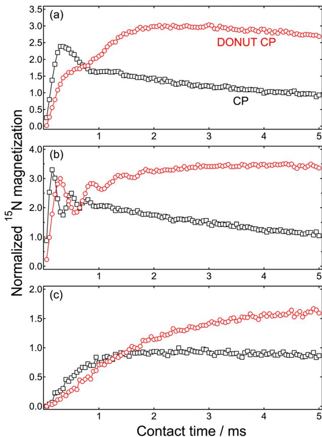
Fig. 6 Contact-time dependence of the  $^{15}\text{N}$  magnetization of (a) the  $\alpha$ , (b) the  $\epsilon_2$  and (c) the  $\delta_1$  sites of  $^{15}\text{N}$ -labeled polycrystalline histidine, measured in a magnetic field of 9.4 T under MAS at 20 kHz by DONUT CP (red circles) and conventional CP (black squares).
