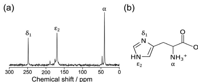
Fig. 5 (a)  $^{15}\text{N}$  spectrum of polycrystalline  $^{15}\text{N}$ -labeled histidine, obtained with DONUT CP in 9.4 T under MAS at 20 kHz with a contact time of 3 ms. (b) The structure of a neutral  $\tau$  tautomer of histidine.
