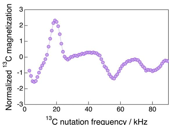
Fig. 4  $^{13}\text{C}$  nutation frequency dependence of methylene  $^{13}\text{C}$  magnetization in 9.5%- $^{13}\text{C}$ -labeled glycine under DONUT CP with  $(\omega_{11}/2\pi, \omega_{21}/2\pi)$  of (90 kHz, 60 kHz) in a magnetic field of 9.4 T under MAS at 23 kHz. The contact time was 0.15 ms.
