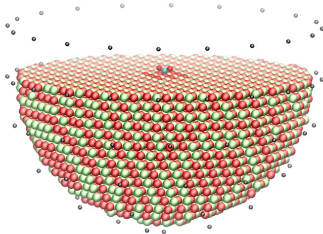
Fig. 5 ChemShell embedded cluster model of CO<sub>2</sub> adsorbed onto an MgO surface. Red spheres = O, green = Mg, cyan = C, black = external point charges.
