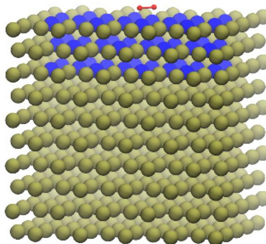
Fig. 6 O<sub>2</sub> (red) adsorbed on the Pd surface optimised using the QM/Me embedding scheme. The 3-layer QM slab is displayed in blue colour.
