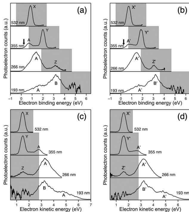
Fig. 2 PE spectra of (a)  $3^{3-}$  and (b)  $4^{3-}$  recorded at 532, 355, 266, and 193 nm plotted against the electron binding energy and PE spectra of (c)  $3^{3-}$  and (d)  $4^{3-}$  plotted against the electron kinetic energy. The gray shaded area is the cutoff region due to the RCB.
