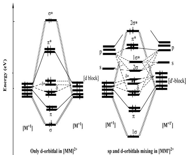
Fig. 4 EHMO diagrams for  $[MM]^{2+}$  (left) and  $[MM']^{2+}$  (right). The wider dashed and the continuous lines indicate the main orbitals involved in the metal–metal bonding. The thin dashed lines indicate the extra-interactions of the  $\sigma$  and  $\sigma^*$  orbitals.
