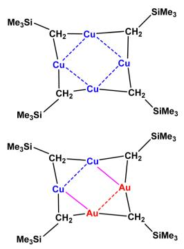
Fig. 3 The experimental molecular structure of the tetranuclear cluster,  $\left[ \mathrm{Cu_4L_4'} \right]$  (4, top), and a proposed mixed-metal analogue,  $\left[ \mathrm{Cu_2Au_2L_2'} \right]$  (5, bottom).
