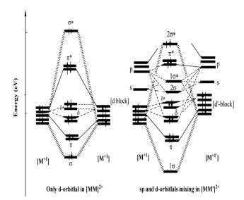
Fig. 4 EHMO diagrams for [MM]<sup>2+</sup> (left) and [MM']<sup>2+</sup> (right). The wider dashed and the continuous lines indicate the main orbitals involved in the metal-metal bonding. The thin dashed lines indicate the extra-interactions of the  $\sigma$  and  $\sigma^*$  orbitals.
