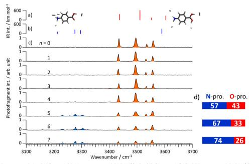
Fig. 5 Calculated IR spectra of the (a) O- and (b) N-protomers of PABAH<sup>+</sup>( $H_2$ )<sub>4</sub>. (c) Observed CAS-IRPD spectra of PABAH<sup>+</sup>( $H_2$ O)<sub>n</sub> (n = 0-7) and (d) estimated population ratio for N- and O-protomers for n = 5-7. The calculated frequencies of the OH stretching modes are overestimated compared to the NH stretching modes
