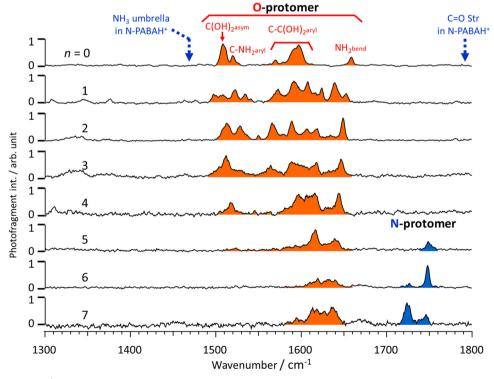
Fig. 2 IRPD spectra of PABAH<sup>+</sup>( $H_2O$ )<sub>n</sub> with n = 0-7.
