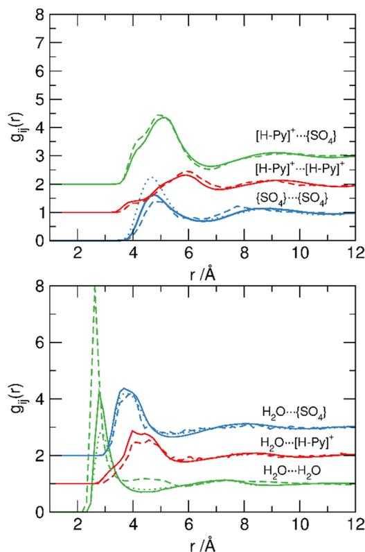
Fig. 3 COM RDFs between  $[\text{H-Py}]^+$  and  $\{\text{SO}_4\}$  (top) and between  $\text{H}_2\text{O}$  and  $[\text{H-Py}]^+$  or  $\{\text{SO}_4\}$  units (bottom) in: concentrated sulfuric acid (dotted lines), Brønsted acidic PIL (solid lines) and hydrated PIL (dashed lines), from the EPSR simulations.
