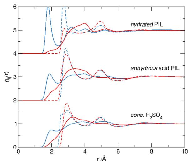
Fig. 5 Site–site pRDFs between water Hw (solid line) and Ow (dashed line) and sulfate  $\text{S}=\text{O}$  (blue) and  $\text{S–OH}$  (red) oxygens in the three systems showing hydrogen-bond donation from the water Hw to the  $\text{S}=\text{O}$  oxygen (1.8 Å) and hydrogen-bond acceptance at Ow from  $\text{S–OH}$  (2.8 Å).
