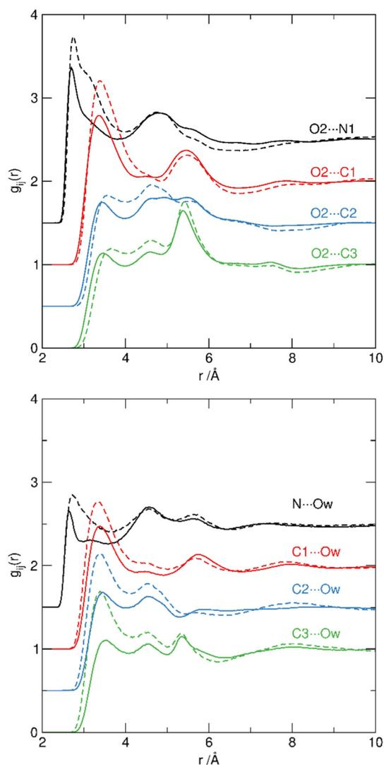
Fig. 7 Site–site RDFs from pyridinium N (black) and C1 (red), C2 (blue) and C3 (green) sites to O2 oxygen atoms of the  $\{\text{SO}_4\}$  units to hydrogensulfate (top) and  $\text{Ow}$  sites in water (bottom) for  $[\text{Hpy}][\text{HSO}_4]\cdot \text{H}_2\text{SO}_4$  (solid lines) and  $[\text{Hpy}][\text{HSO}_4]\cdot 2\text{H}_2\text{O}$  (dashed). Each set of correlations is displaced by 0.5 in the y-axis for clarity.
