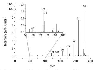
Fig. 3 Cumulative MS for the  $m/z=229~{\rm Cys(H_2O)_6}^+$  precursor ion created as a sum of individual CID MS in counts per second obtained at lab frame energies of (8, 11, 16, 21, 26, 31, 36, 46, 56, 66, 76, 86, 96, and 106) eV.
