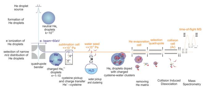
Fig. 1 Schema of the experiment.
