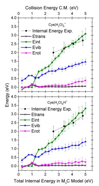
Fig. 8 Distribution of the energy transferred to the cluster degrees of freedom upon collision-induced activation as a function of the internal energy of the  $Cys(H_2O)_6^+$  (top) and  $Cys(H_2O)_6H^+$  (bottom) cluster cations calculated using the  $M_3C$  approach. The black squares represent the mean value of the internal energy distributions obtained by fitting the experimental mass spectra (see Fig. 9).
