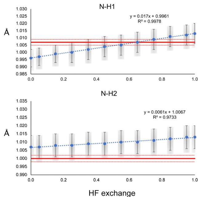
Fig. 2 N–H1 and N–H2 distances refined with the HAR for different percentages of HF exchange with the  $\text{PBE}_x$  functional and the def2-TZVP basis set. The red line corresponds to the neutron diffraction value. The least-squares std errors of the HAR and neutron diffraction are shown as blue bars and red dashed lines, respectively.
