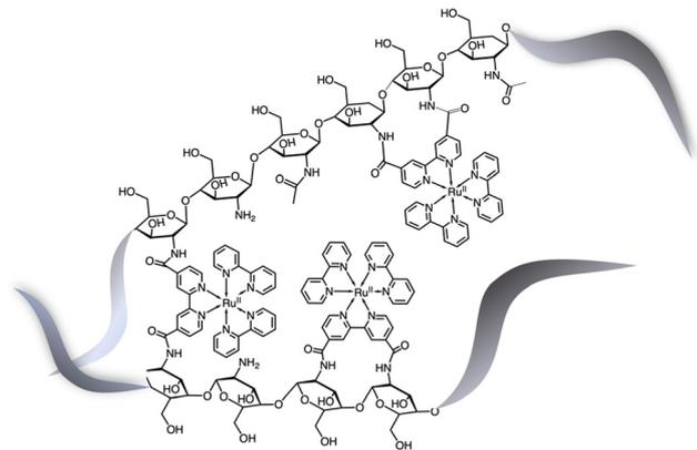
Fig. 11 Schematization of the structural formula of the chitosan polymer containing the Ru(II) chromophores.<sup>25</sup> The metal complexes are linked to the polysaccharide framework exclusively by chitosan–N(H)–C(O)–bipyridine connections.
