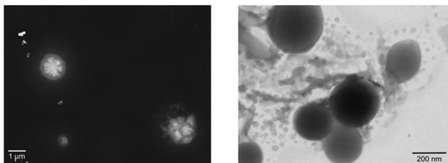
Fig. 5 STEM image obtained from (left, registered in annular dark field-ADF)  $5 \times 10^{-6}$  M and from (right, registered in bright field-BF)  $5 \times 10^{-5}$  M acetonitrile solution of **OsRu9**.
