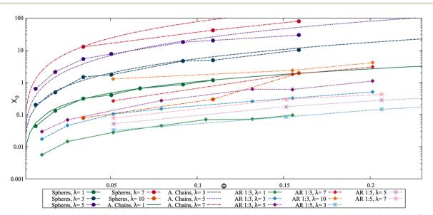
Fig. 16 Initial magnetic susceptibilities (y-axis) at different volume fractions (x-axis): analytical approximations for spheres (dashed lines), simulation values for spheres (dark colors with circular points), simulation values for aspect ratio 1:3 platelets (medium colors, rhombi) and aspect ratio 1:5 platelets (light colors, stars). We see that platelets have lower magnetic susceptibilities that their spherical equivalents.
