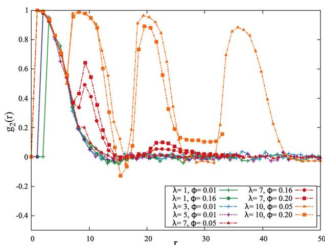
Fig. 12 Pairwise orientational correlation of aspect ratio 1:3 platelets, where the  $x$ -axis indicates the radial distance and the  $y$ -axis is the pairwise orientational correlation. We note a much stricter alignment at close distances due to the steric repulsion, as well as more pronounced peaks for the higher  $\lambda$  systems.
