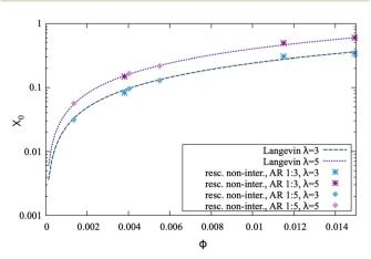
Fig. 17 Langevin curves for two different values of  $\lambda$ , as well simulations results for non-interacting platelets at rescaled densities. If the densities are rescaled to match the equivalent sphere system, and magnetic interparticle interactions are disabled, platelets follow the Langevin law.
