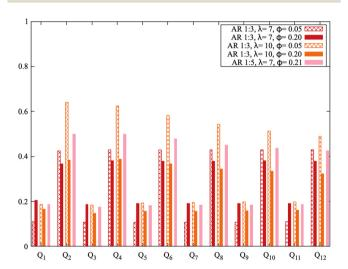
**Fig. 15** Steinhardt Bond order parameters for platelets of aspect ratio 1:3 (red and orange curves) and 1:5 (pink curve),  $Q_1$  through  $Q_{12}$ . We see that the even Q values are significantly higher than the odds, especially for higher  $\lambda$ . Moreover, at high  $\lambda$  and low density these peaks easily surpass their equivalents in dipolar sphere systems.
