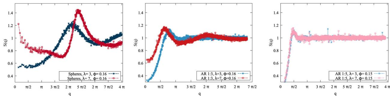
Fig. 5 Structure factors  $S(q)$  of spheres (left), aspect ratio 1:3 platelets (center) and aspect ratio 1:5 platelets at density  $\phi = 0.15$ , with  $\lambda = 3$  (blue, stars) and  $\lambda = 7$  (red, hollow squares). While the spheres show a pronounced structuring that is strongly affected by  $\lambda$ , only aspect ratio 1:3 platelets with high  $\lambda$  show structure beyond that of a homogeneous fluid.
