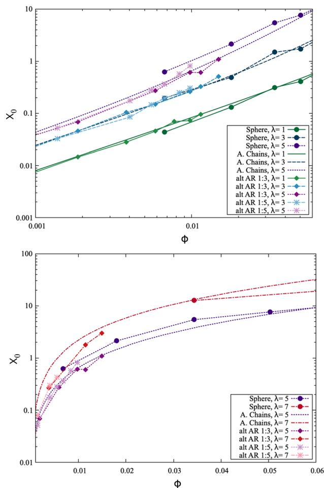
Fig. 18 Initial susceptibilities of magnetic platelets and spheres, shown with a rescaled volume fraction for platelets. We see excellent agreement for the lower values of  $\lambda$  (blue and green curves, top plot), while at higher  $\lambda$ , the initial magnetic susceptibilities appear to follow a steeper progression than spheres and still appear lower than theoretical predictions.
