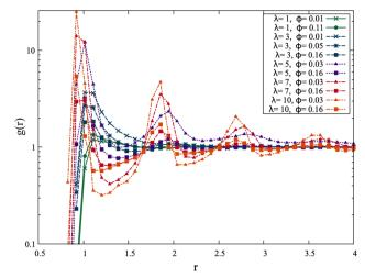
Fig. 2 Radial distribution functions g(r) of dipolar sphere particles for varying magnetic coupling  $\lambda$  and volume fraction  $\phi$ . We observe initial gaseous states for low  $\lambda$  (green), followed by some form of self-assembly for all higher values of magnetic moment. At high  $\lambda$  and high  $\phi$ , we see the most pronounced structuring with peaks and valleys persisting at longer ranges.
