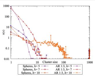
Fig. 8 The average number of particles n in clusters of size s, normalized by the number of checkpoints, shown for the fixed densities  $\phi$  = 0.03 (spheres) and  $\phi$  = 0.16 (aspect ratio 1:3 platelets). The systems of dipolar spheres (lines with circular points) agree with the Wertheim theory, systems of platelets (stars) either do not cluster sufficiently (purple) or strongly diverge from any expected power law (orange).
