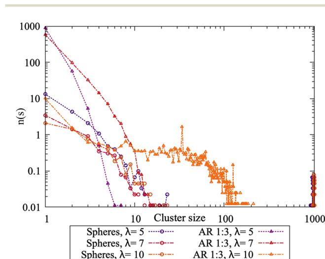
**Fig. 8** The average number of particles  $n$  in clusters of size  $s$ , normalized by the number of checkpoints, shown for the fixed densities  $\phi = 0.03$  (spheres) and  $\phi = 0.16$  (aspect ratio 1:3 platelets). The systems of dipolar spheres (lines with circular points) agree with the Wertheim theory, systems of platelets (stars) either do not cluster sufficiently (purple) or strongly diverge from any expected power law (orange).
