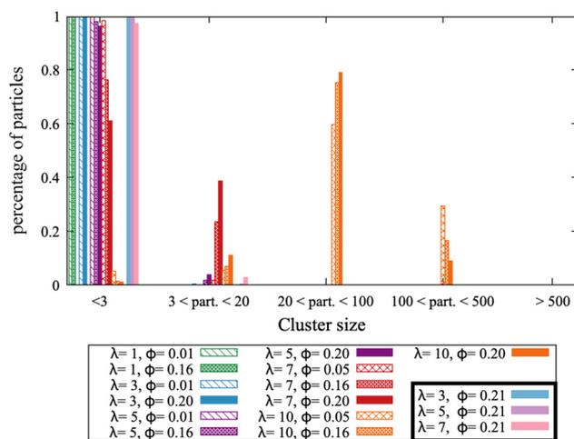
Fig. 7 Histogram depicting the percentage of aspect ratio 1:3 (bright colors) and aspect ratio 1:5 (pastel colors, black box in legend) particles in a cluster of size  $n$ . We see that clusters only form for high values of  $\lambda$  (orange and red), and that none of the large clusters observed as high  $\lambda$ ,  $\phi$  limit for spheres are formed.
