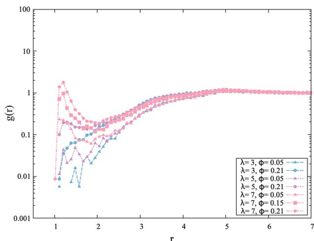
Fig. 4 Radial distribution functions  $g(r)$  of aspect ratio 1:5 particles for a reduced set of magnetic coupling parameters  $\lambda \in \{3, 5, 7\}$  and volume fractions  $\phi$ . We observe initial gaseous states for essentially all  $\lambda$  (light blue, light purple, pink) with a suggestion of a peak for the highest density and  $\lambda$  shown (pink polygons).
