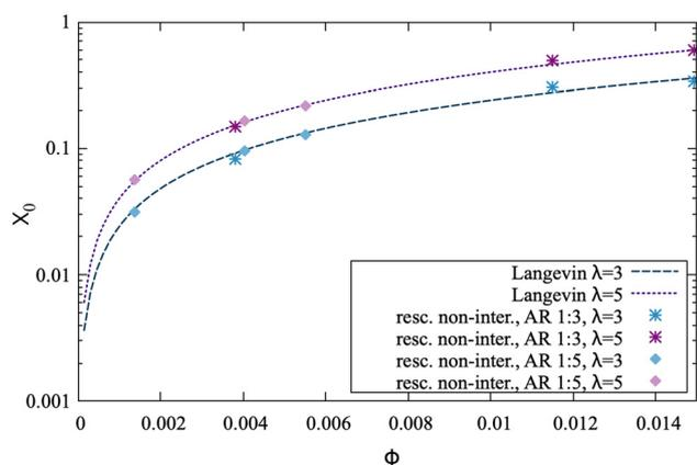
Fig. 17 Langevin curves for two different values of  $\lambda$ , as well simulation results for non-interacting platelets at rescaled densities. If the densities are rescaled to match the equivalent sphere system, and magnetic interparticle interactions are disabled, platelets follow the Langevin law.
