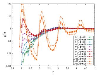
Fig. 3 Radial distribution functions g(r) of aspect ratio 1:3 particles for varying magnetic coupling  $\lambda$  and volume fraction  $\phi$ . We observe initial gaseous states for low  $\lambda$  (blue, green, purple), some clustering for  $\lambda = 7$  at high  $\phi$  (red, square and polygonal points) and the formation of long chains at very high  $\lambda$  (orange).
