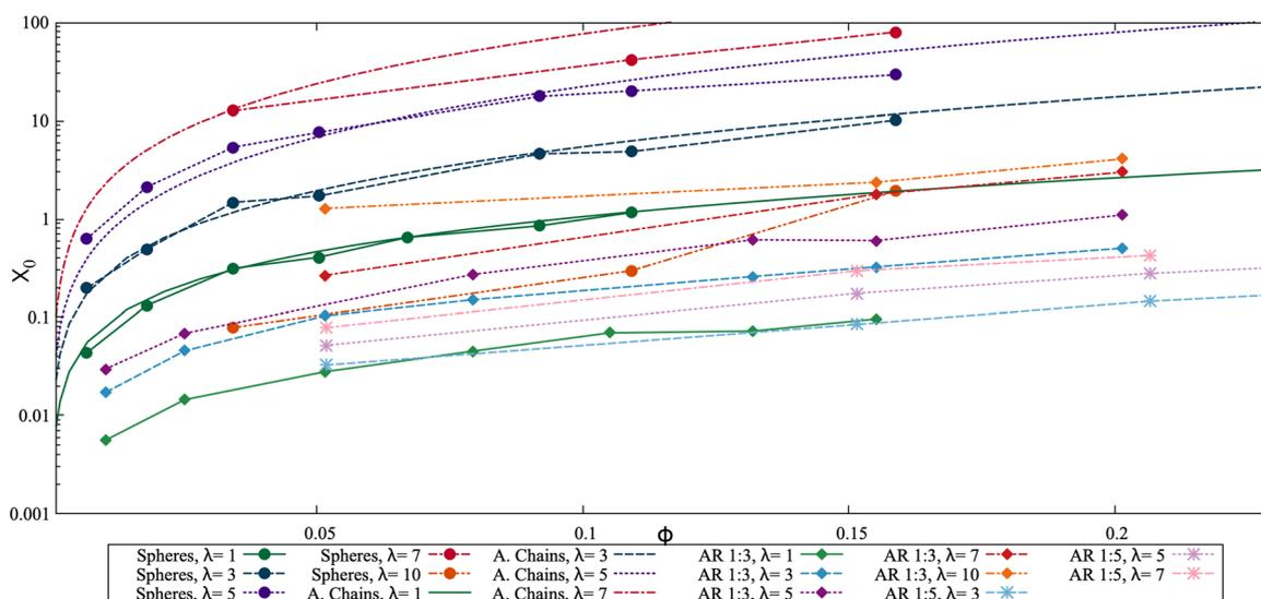
Fig. 16 Initial magnetic susceptibilities ( $y$ -axis) at different volume fractions ( $x$ -axis): analytical approximations for spheres (dashed lines), simulation values for spheres (dark colors with circular points), simulation values for aspect ratio 1:3 platelets (medium colors, rhombi) and aspect ratio 1:5 platelets (light colors, stars). We see that platelets have lower magnetic susceptibilities than their spherical equivalents.
