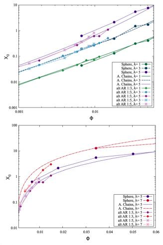
Fig. 18 Initial susceptibilites of magnetic platelets and spheres, shown with a rescaled volume fraction for platelets. We see excellent agreement for the lower values of  $\lambda$  (blue and green curves, top plot), while at higher  $\lambda$ , the initial magnetic suscepibilities appear to follow a steeper progression than spheres and still appear lower than theoretical predictions.
