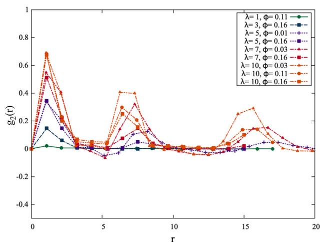
**Fig. 11** Pairwise orientational correlation of spheres, where the  $x$ -axis indicates the radial distance and the  $y$ -axis is the pairwise orientational correlation, ranging from perfectly aligned at 1 to negatively correlated at  $-0.5$ . We observe that the correlations peak at positions where the neighbors in an assembled structure would be located.
