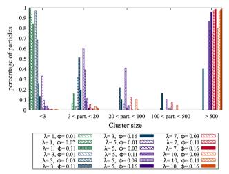
Fig. 6 Histogram depicting the percentage of spheres in a cluster with nparticles. The color indicates the value of  $\lambda$ , the fill indicates the volume fraction  $\phi$ . We see that increasing the value of  $\lambda$  (warmer colors) or increasing  $\phi$  (more filled bars) leads to the majority of particles being contained in larger clusters.
