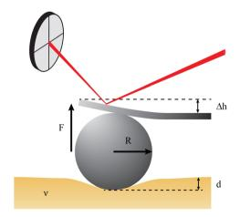
Fig. 4 Example measurement of elastic properties using AFM. A material of known Poisson's ratio  $\nu$  is indented by a sphere of radius R attached to an AFM cantilever. The cantilever has a spring constant of k (calculated before the experiment), and is bent by a distance  $\Delta h$ , indicating a force  $|\mathbf{F}| = k\Delta h$ . Applying the Hertz model from eqn (16), the Young's modulus is calculated as  $E = \frac{3F}{4\sqrt{R}} \frac{(1-\nu^2)}{d^{3/2}}$ .
