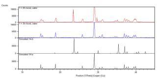
Fig. 1 PXRD pattern of 1 sublimed with 20  $\mu L$  water (red) and 30  $\mu L$ water (blue), compared to simulated patterns (black) for the anhydrous and hydrate crystals.
