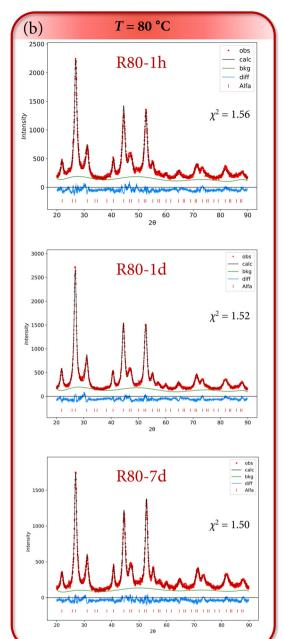
Fig. 5 Rietveld refinements of the XRD patterns for samples obtained at (a) 60 °C and (b) 80 °C. The goodness of fit  $\chi^2$  parameter is also indicated in each plot.
