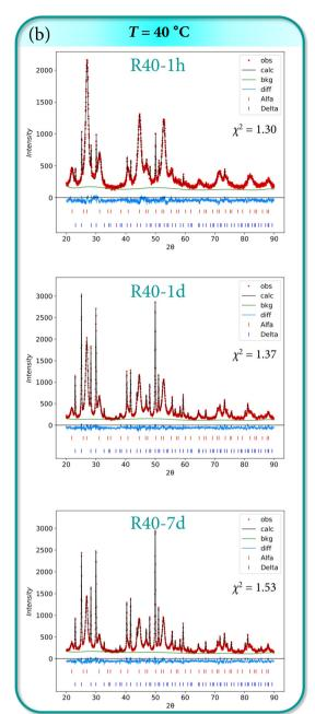
Fig. 4 Rietveld refinements of the XRD patterns for samples obtained at (a) 25 °C and (b) 40 °C. The goodness of fit  $\chi^2$  parameter is also indicated in each plot.
