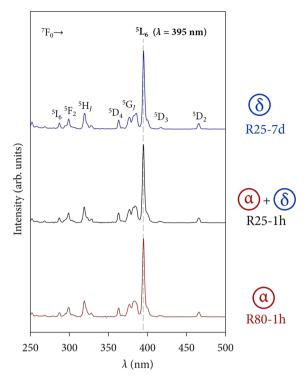
Fig. 9 Room temperature excitation spectra obtained with a DT = 0.2 ms for different samples as an example of the  $\delta$ -phase,  $\alpha$ -phase, and  $\alpha$ +  $\delta$ . The dashed line at 395 nm serves as a guideline to observe that there are no substantial changes in the excitation spectra of the different powders and the maximum intensity corresponds to the band associated with the  $^7F_0 \rightarrow ^5L_6$  transition (395 nm).
