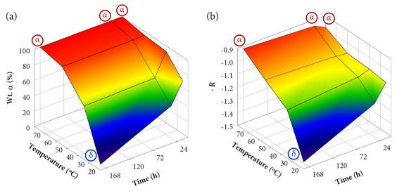
Fig. 11 3D plots of (a) the weight fractions of  $\alpha$ -KY<sub>3</sub>F<sub>10</sub> and (b) the negation of the asymmetry ratio as a function of temperature and time. For samples that exhibit a single  $\delta$ -phase (R25-7 d) or single  $\alpha$ -phase (R80-1 h, R80-1 d, R80-7 d), the label " $\alpha$ " or " $\delta$ " has been added as an inset in the corresponding point.
