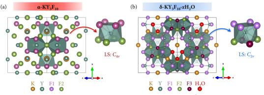
Fig. 1 Structure of (a)  $\alpha$ -KY<sub>3</sub>F<sub>10</sub> and (b)  $\delta$ -KY<sub>3</sub>F<sub>10</sub>·xH<sub>2</sub>O highlighting the coordination polyhedra of Y<sup>3+</sup> ions along with their local symmetry. The labels F1, F2, and F3 refer to fluoride anions situated at different Wyckoff positions in each compound. The global structure view has been selected for simplification proposes due to the high number of atoms.
