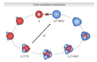
Fig. 6 Schematic representation of the suggested cross-nucleation mechanism that explains the obtention of the metastable  $\delta$ -phase instead of the thermodynamic  $\alpha$ -phase when exposing the precipitate  $(\alpha + \delta)$  at long times of maturing.  $t_m$  indicates an intermediate time of maturing
