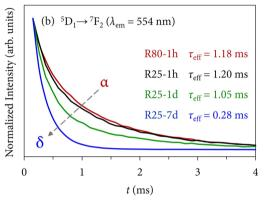
**Fig. 12** Normalized decay curves acquired at room temperature with a DT = 0.2 ms exciting the samples at 395 nm and collecting the emission at (a) 593 nm ( $^5D_0 \rightarrow {}^7F_1$  transition) for the lowest-lying excited state  $^5D_0$ , and (b) 554 nm ( $^5D_1 \rightarrow {}^7F_2$  transition) for the higher excited state  $^5D_1$ .
