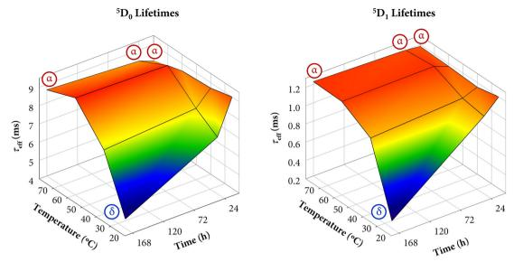
**Fig. 13** 3D plot of the lifetimes corresponding to the  $^5D_0$  and  $^5D_1$  states as a function of temperature and time. For samples that exhibit a single δ-phase (R25-7 d) or single α-phase (R80-1 h, R80-1 d, R80-7 d), the label " $\alpha$ " or " $\delta$ " has been added as an inset in the corresponding point.
