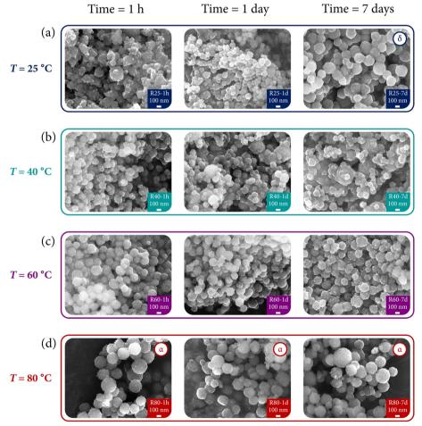
Fig. 7 SEM images of the Eu<sup>3+</sup>-doped powders prepared under different reaction conditions of time and temperature: (a) compounds prepared at 25 °C, (b) compounds prepared at 40 °C, (c) compounds prepared at 60 °C, and (d) compounds prepared at 80 °C. For samples that exhibit a single  $\delta$ -phase (R25-7 d) or single  $\alpha$ -phase (R80-1 h, R80-1 d, R80-7 d), the label " $\alpha$ " or " $\delta$ " has been added as an inset in the corresponding micrograph.
