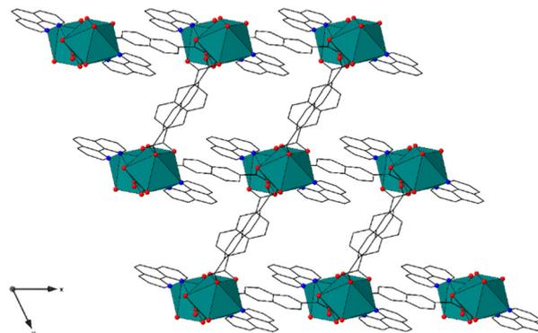
Fig. 3 The structure of **LP-3** is three-dimensional. The channels contain noncoordinated DMF guest species, which are not shown for clarity.
