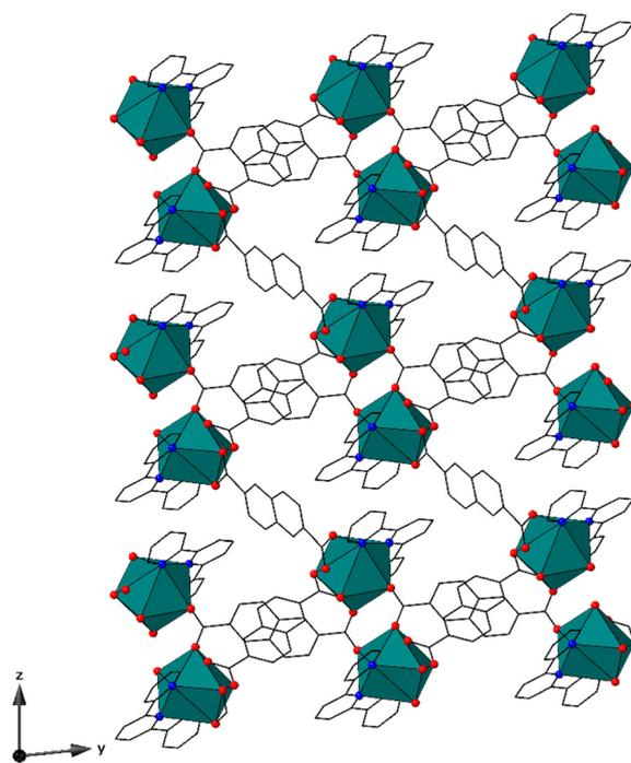
**Fig. 1** The structure of **LP-1** is three-dimensional and contains small pores that propagate along the [100] direction. The  $\text{Eu}^{3+}$  atoms are drawn as teal polyhedra. The O and N atoms are depicted as red and blue spheres, respectively, and the C atoms are represented by black sticks. The H atoms and solvent water molecules are omitted for clarity here and throughout this manuscript.
