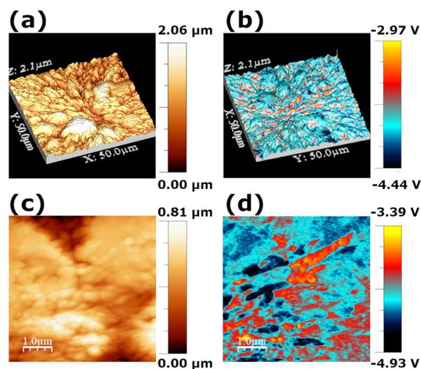
Fig. 6 AFM images of [4PyAla][BF<sub>4</sub>] sample. (a) Topography (3D view); (b) topography with OOP piezoresponse (3D view); (c) topography (2D view); (d) topography with piezoresponse (2D view).
