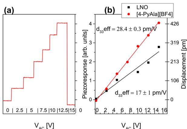
Fig. 7 (a) OOP piezoresponse of [4PyAla][BF<sub>4</sub>] vs. driving voltage. (b) Driving voltage dependence of OOP piezoresponse of LNO and [4PyAla][BF<sub>4</sub>].
